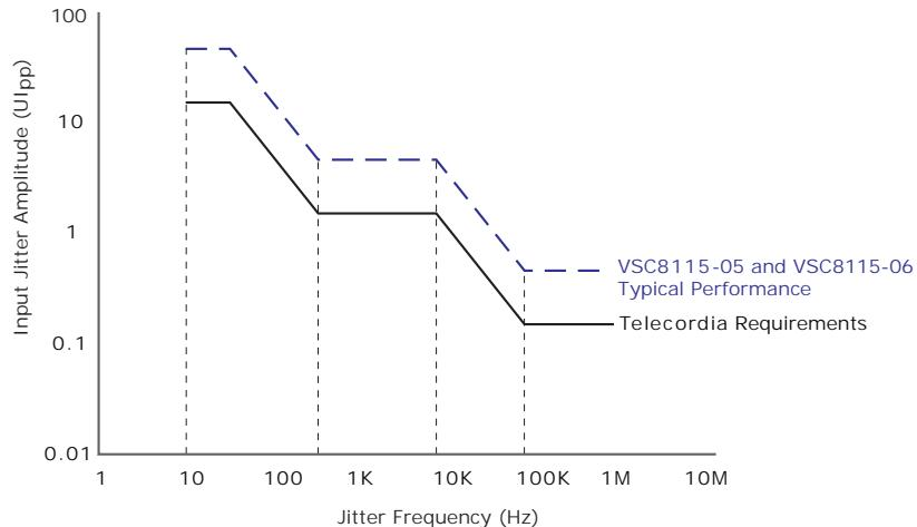
OC-12 Jitter Tolerance Minimum Specifications
