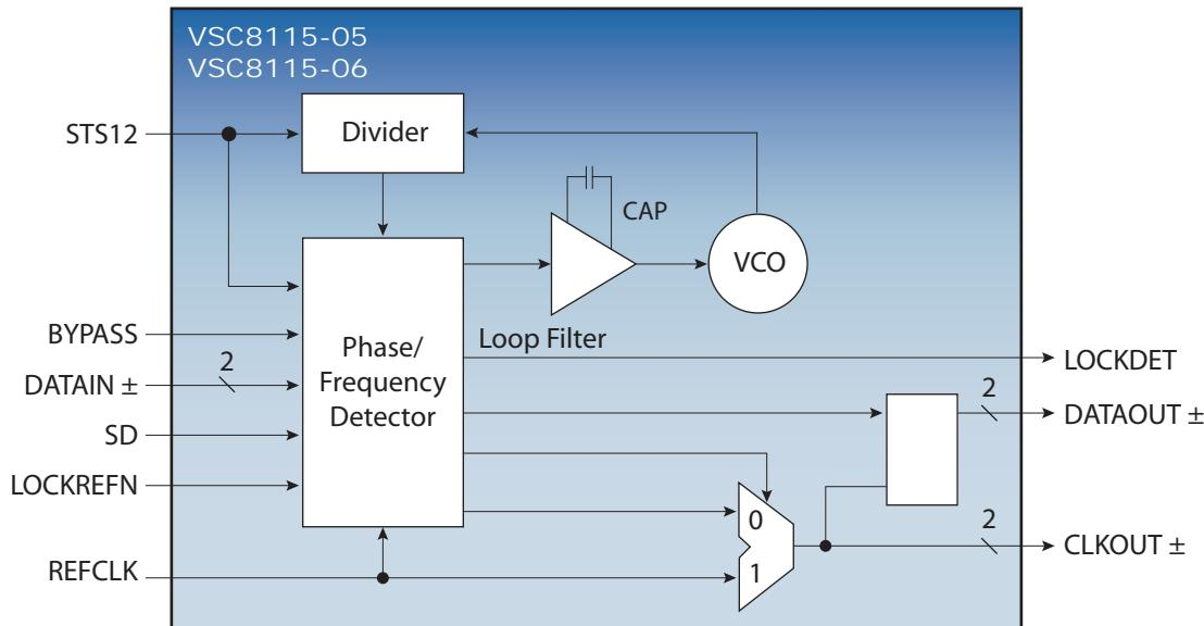
Use the VSC8115-05 or VSC8115-06 for OC-12 (STM-4) and OC-3 (STM-1) NRZ data clocking and recovery.
