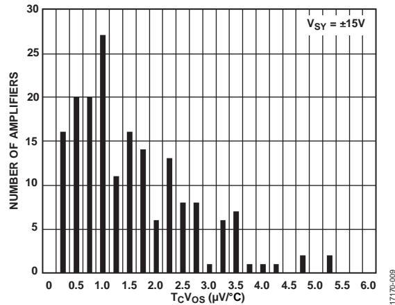
Figure 3.  $T_c V_{OS}$  Distribution
