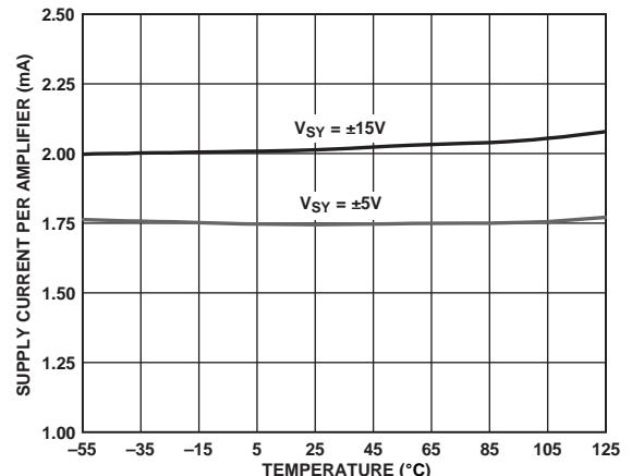
Figure 6. Supply Current per Amplifier vs. Temperature
