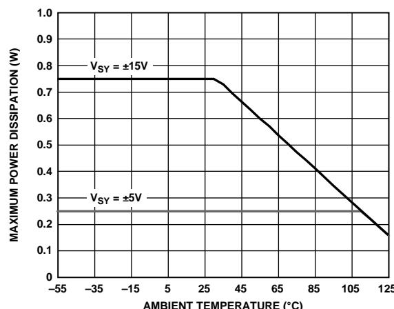
Figure 2. Maximum Power Dissipation vs. Ambient Temperature
