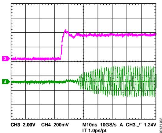
Figure 35. DSA: Gain Settling Time, 31.5 dB to 0 dB
