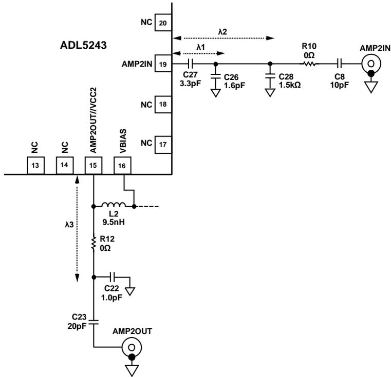
Figure 67. AMP2: Matching Circuit at 2350 MHz
