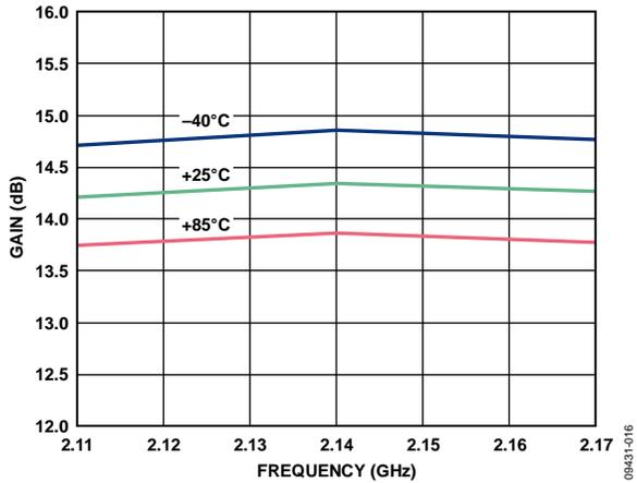
Figure 16. AMP2-2140 MHz: Gain vs. Frequency and Temperature
