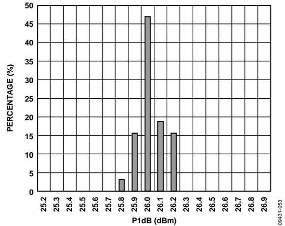
Figure 55. AMP2: P1dB Distribution at 2140 MHz
