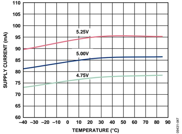
Figure 48. AMP2: Supply Current vs. Voltage and Temperature
