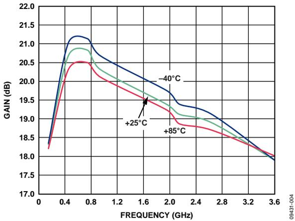
Figure 4. AMP1: Gain vs. Frequency and Temperature
