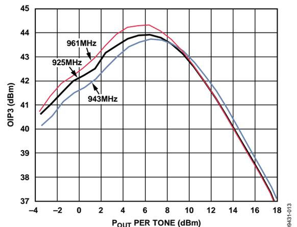
Figure 13. AMP2-943 MHz: OIP3 vs.  $P_{OUT}$  and Frequency
