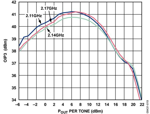
Figure 19. AMP2-2140 MHz: OIP3 vs.  $P_{OUT}$  and Frequency
