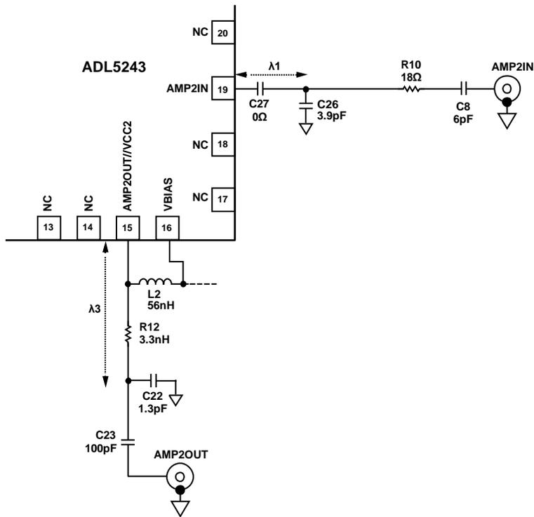
Figure 64. AMP2: Matching Circuit at 943 MHz
