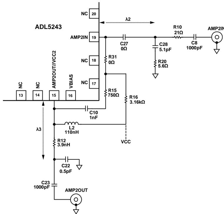
Figure 62. AMP2: Matching Circuit at 450 MHz
