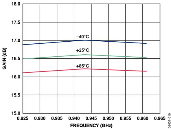
Figure 10. AMP2-943 MHz: Gain vs. Frequency and Temperature
