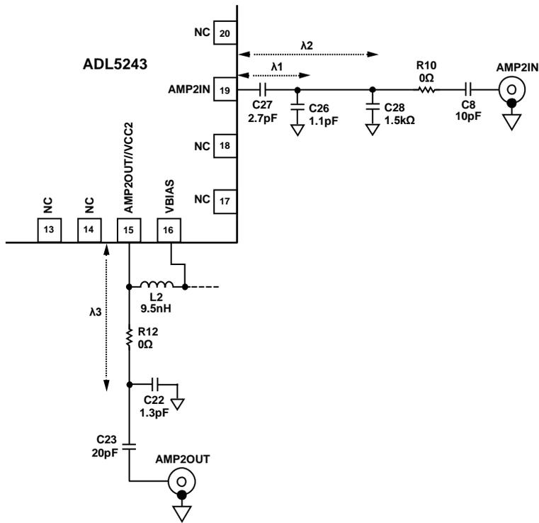
Figure 68. AMP2: Matching Circuit at 2630 MHz
