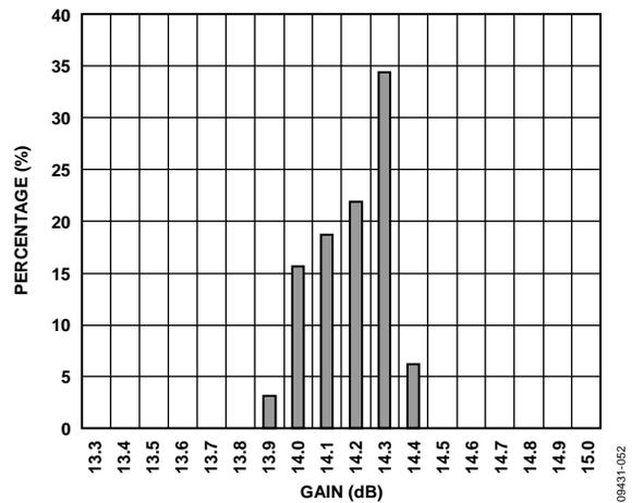
Figure 54. AMP2: Gain Distribution at 2140 MHz
