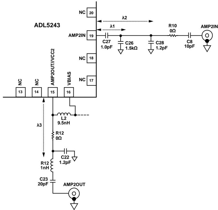
Figure 69. AMP2: Matching Circuit at 3600 MHz
