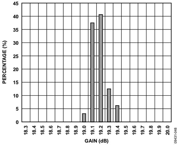
Figure 50. AMP1: Gain Distribution at 2140 MHz
