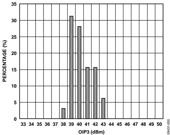
Figure 52. AMP1: OIP3 Distribution at 2140 MHz
