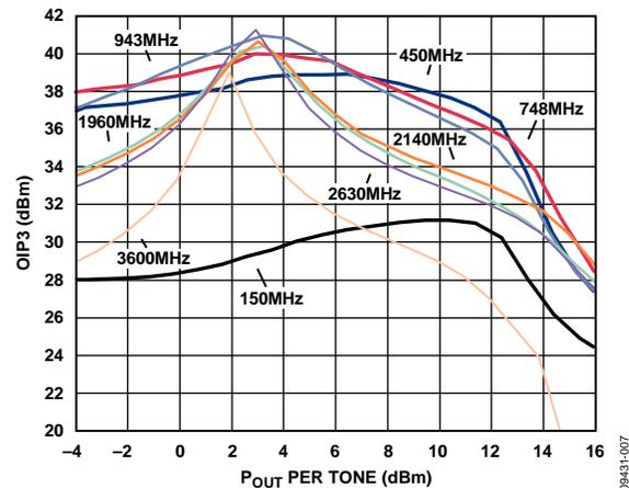
Figure 7. AMP1: OIP3 vs.  $P_{OUT}$  and Frequency
