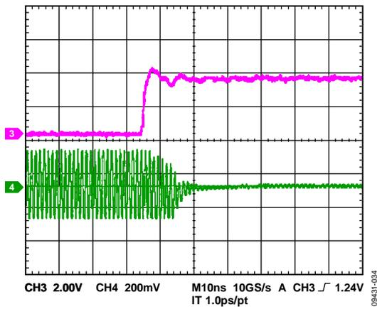
Figure 34. DSA: Gain Settling Time, 0 dB to 31.5 dB
