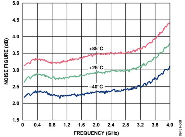
Figure 8. AMP1: Noise Figure vs. Frequency and Temperature
