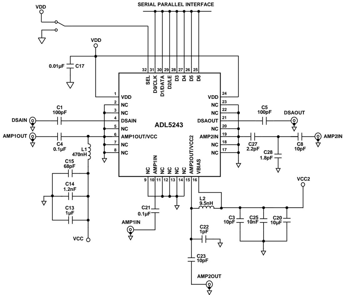
Figure 58. Basic Connections
