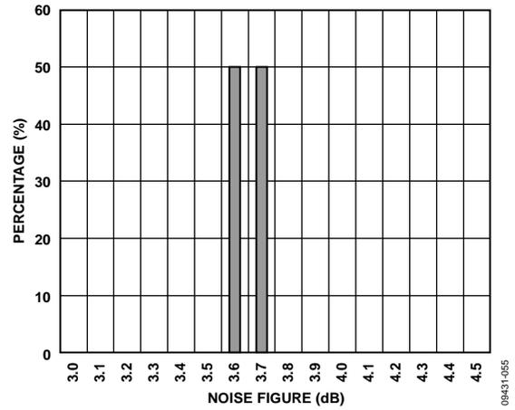
Figure 57. AMP2: Noise Figure Distribution at 2140 MHz
