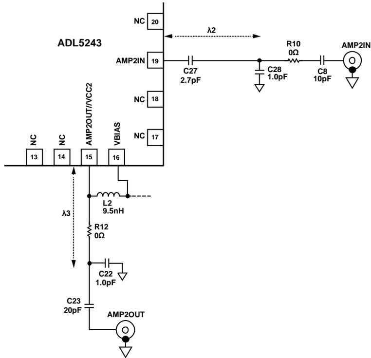
Figure 65. AMP2: Matching Circuit at 1960 MHz
