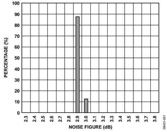
Figure 53. AMP1: Noise Figure Distribution at 2140 MHz
