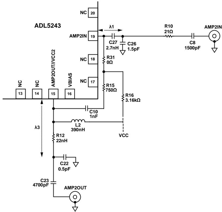
Figure 61. AMP2: Matching Circuit at 150 MHz
