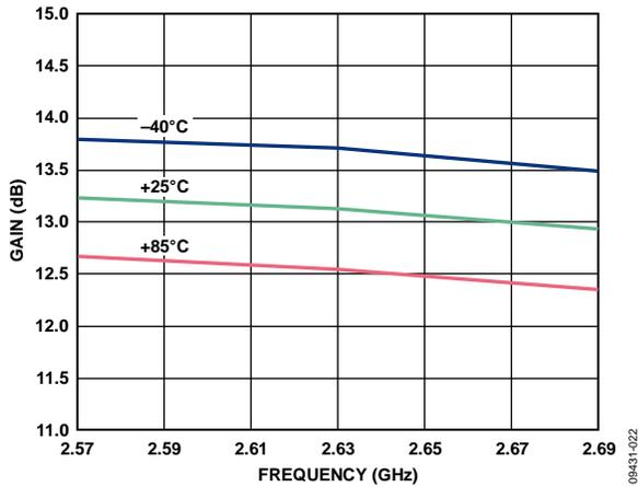
Figure 22. AMP2-2630 MHz: Gain vs. Frequency and Temperature
