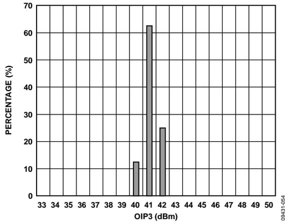
Figure 56. AMP2: OIP3 Distribution at 2140 MHz
