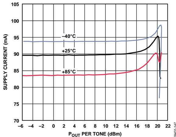
Figure 47. AMP1: Supply Current vs.  $P_{OUT}$  and Temperature
