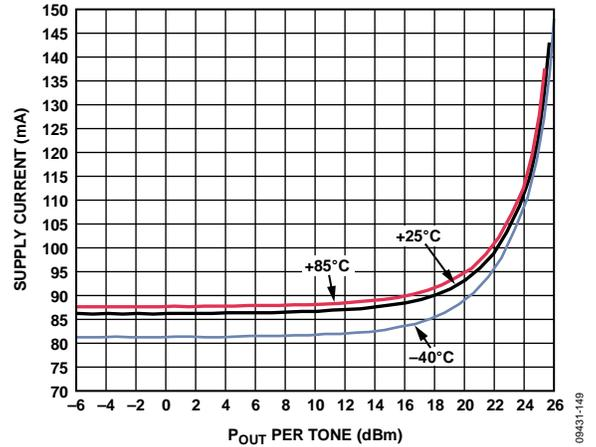
Figure 49. AMP2: Supply Current vs.  $P_{OUT}$  and Temperature
