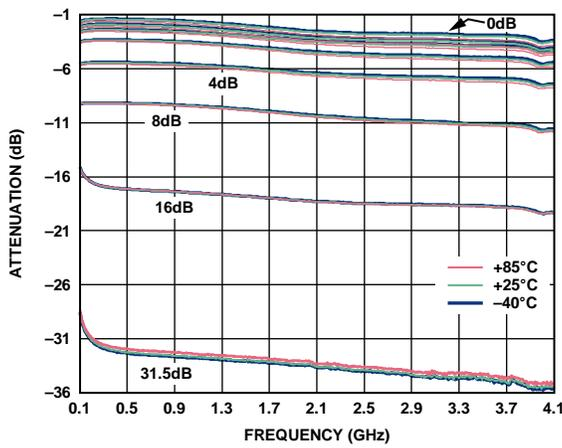
Figure 28. DSA: Attenuation vs. Frequency and Temperature
