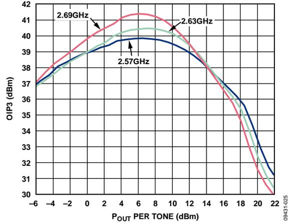
Figure 25. AMP2-2630 MHz: OIP3 vs.  $P_{OUT}$  and Frequency
