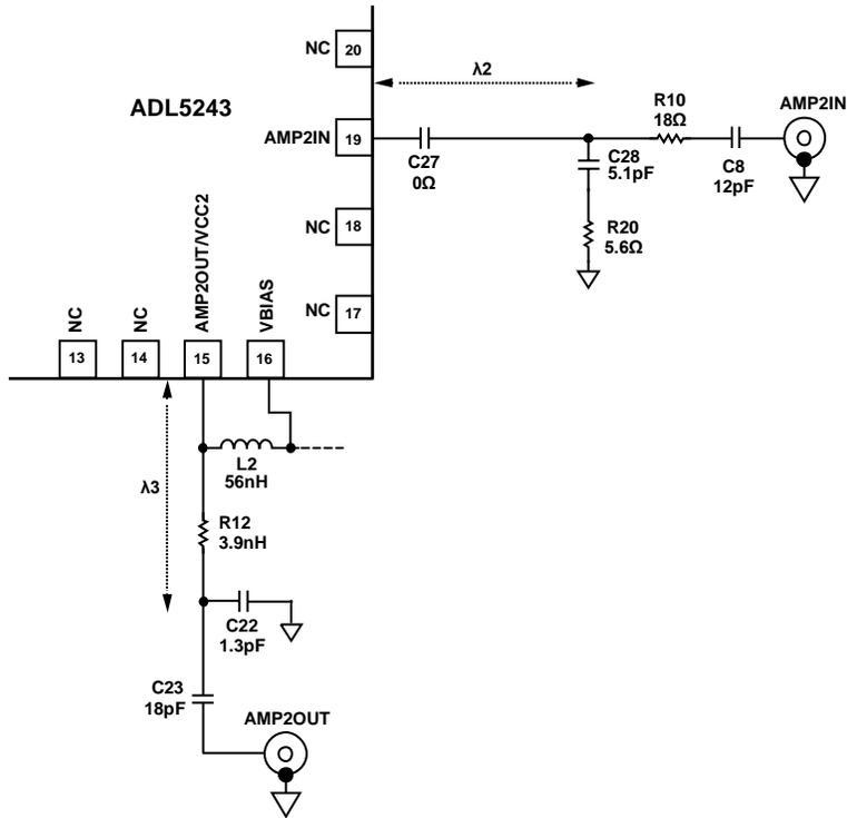
Figure 63. AMP2: Matching Circuit at 748 MHz
