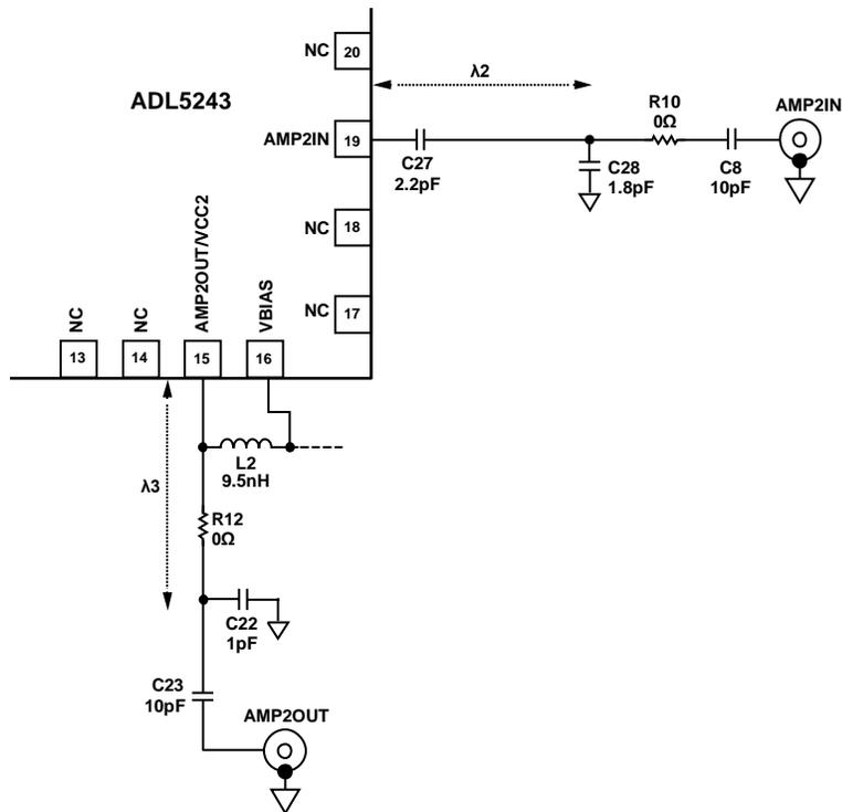
Figure 66. AMP2: Matching Circuit at 2140 MHz
