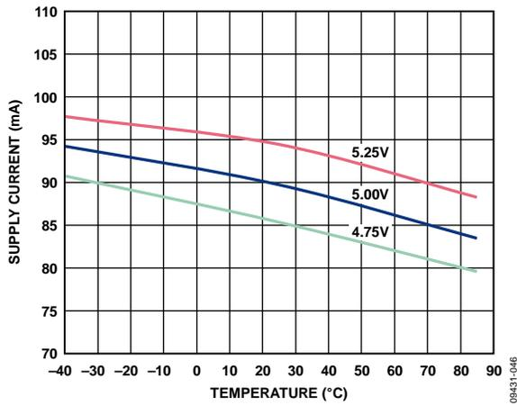
Figure 46. AMP1: Supply Current vs. Voltage and Temperature
