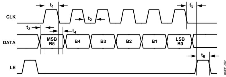
Figure 59. SPI Timing Diagram (Data Loaded MSB First)
