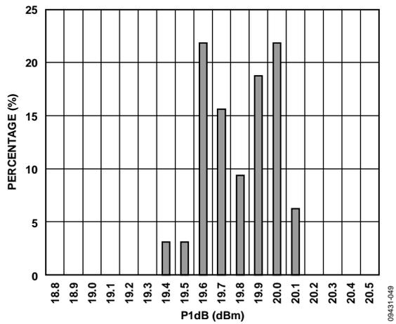
Figure 51. AMP1: P1dB Distribution at 2140 MHz
