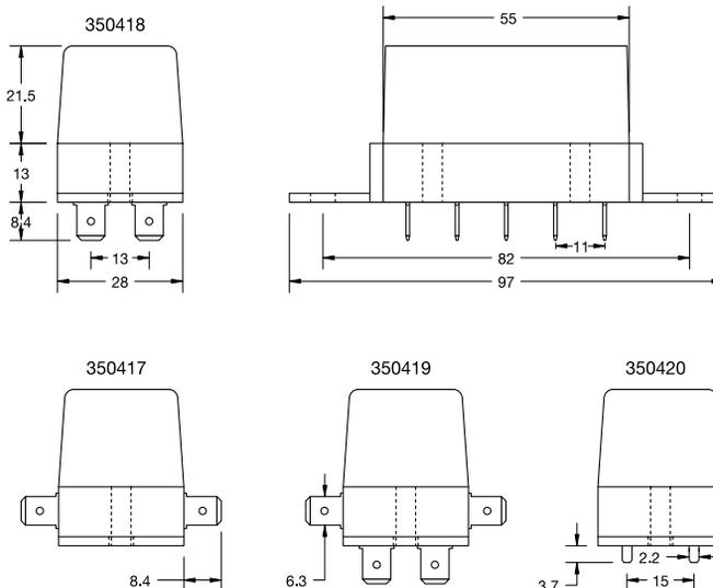
Use with ATO fuses up to 15A. Available in 5 pole unit with removable clear protective cover. Available in side or bottom positioned 1/4" Q.C. terminal configurations. Unit with bottom Q.C. terminals includes detachable side mounting brackets.
