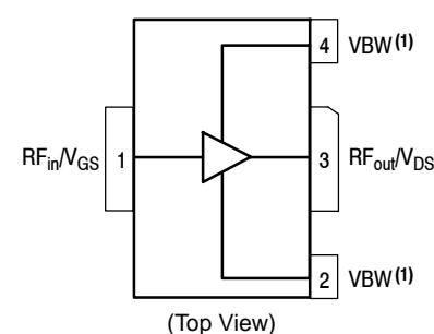
Figure 1. Pin Connections
