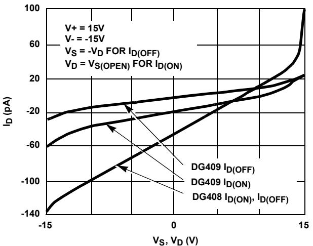
FIGURE 15. DRAIN LEAKAGE CURRENT vs SOURCE/DRAIN VOLTAGE
