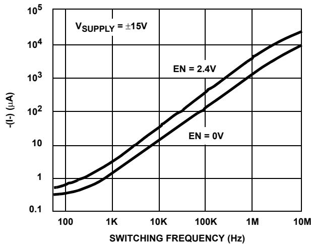
FIGURE 18. NEGATIVE SUPPLY CURRENT vs SWITCHING FREQUENCY
