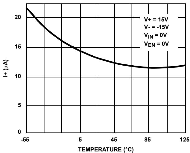
FIGURE 22. POSITIVE SUPPLY CURRENT vs TEMPERATURE (DG408)
