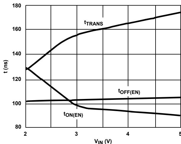
FIGURE 32. SWITCHING TIME vs V<sub>IN</sub> (BIPOLAR SUPPLY)
