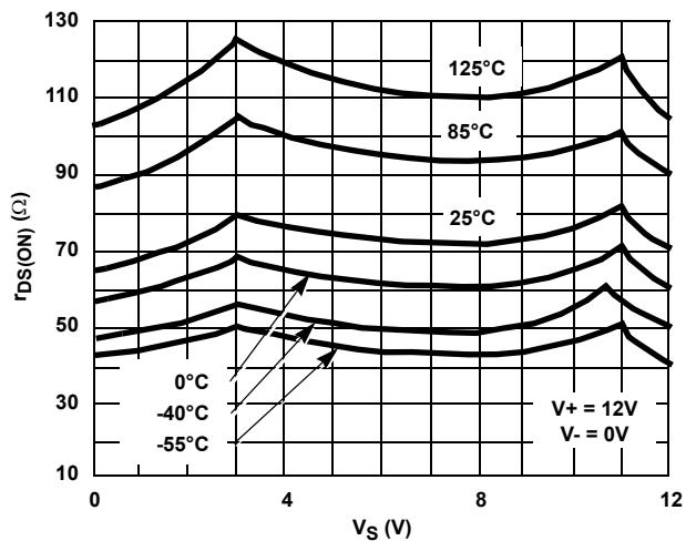
FIGURE 27.  $r_{\text{DS(ON)}}$  vs  $V_S$  AND TEMPERATURE (SINGLE SUPPLY)
