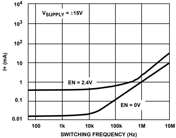
FIGURE 19. POSITIVE SUPPLY CURRENT vs SWITCHING FREQUENCY
