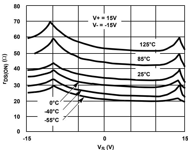
FIGURE 26.  $r_{\text{DS(ON)}}$  vs  $V_S$  AND TEMPERATURE
