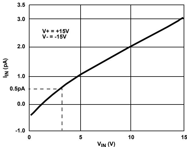
FIGURE 10. INPUT LOGIC CURRENT vs LOGIC INPUT VOLTAGE
