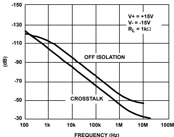
FIGURE 28. OFF ISOLATION AND CROSSTALK vs FREQUENCY
