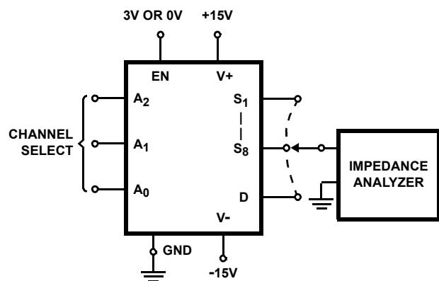
FIGURE 8. SOURCE/DRAIN CAPACITANCES
