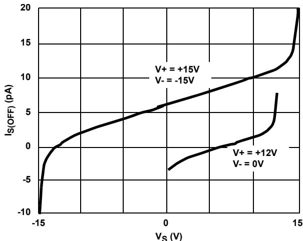
FIGURE 16. SOURCE LEAKAGE CURRENT vs SOURCE VOLTAGE
