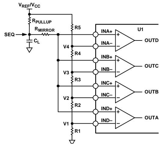
Figure 34. Circuit Configuration for a Mirrored Voltage Sequencer
