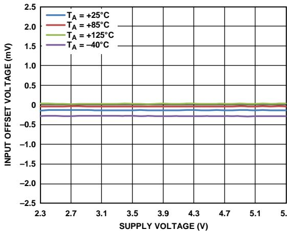
Figure 11. Input Offset Voltage ( $V_{os}$ ) vs. Supply Voltage ( $V_{cc}$ ),  $V_{cm} = 1\text{ V}$
