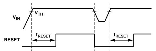
Figure 37. Threshold and Timeout Programmable Voltage Supervisor Timing Diagram
