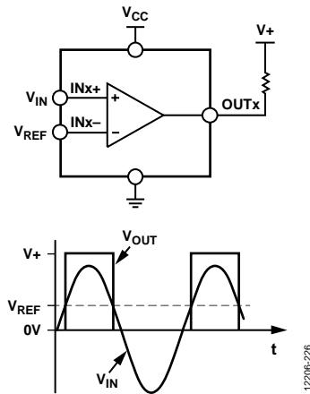
Figure 26. Basic Comparator and Input and Output Signals
