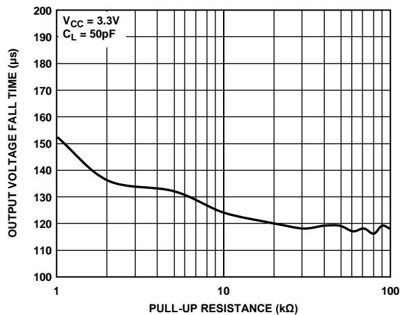
Figure 25. Output Voltage Fall Time ( $t_f$ ) vs. Pull-Up Resistance ( $R_{PULLUP}$ )
