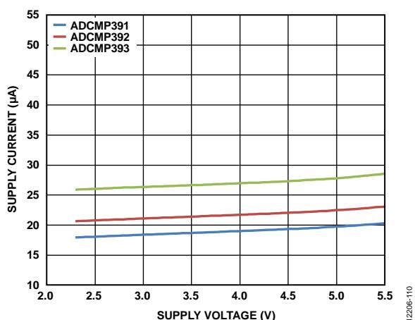
Figure 10. Supply Current vs. Supply Voltage ( $V_{cc}$ ) at Output Low Voltage
