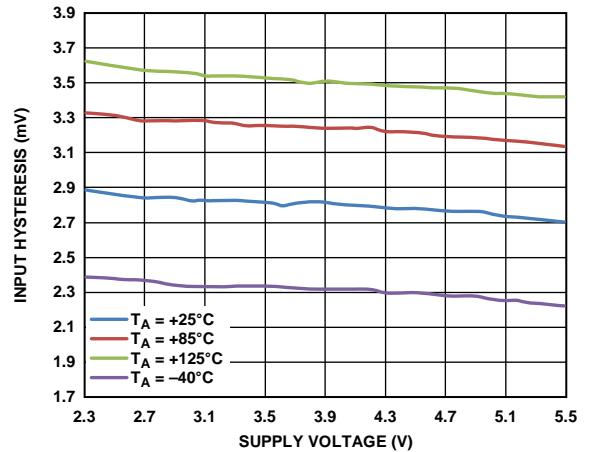
Figure 18. Input Hysteresis vs. Supply Voltage ( $V_{CC}$ ) for Various Temperatures,  $V_{CM} = 1\text{ V}$
