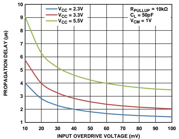
Figure 23. Propagation Delay vs. Input Overdrive Voltage, High to Low
