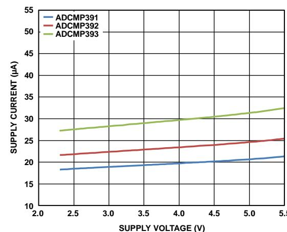
Figure 13. Supply Current vs. Supply Voltage ( $V_{cc}$ ) at Output High Voltage
