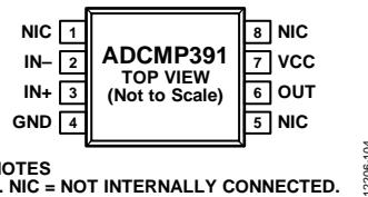
Figure 4. *ADCMP391 Pin Configuration*
