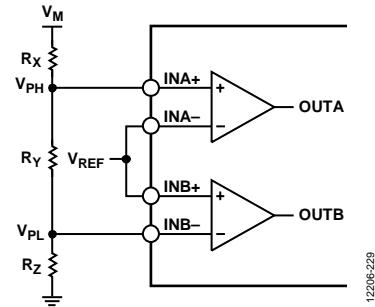
Figure 29. Positive Undervoltage/Ovvoltage Monitoring Configuration
