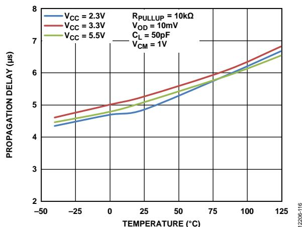
Figure 16. Propagation Delay vs. Temperature, Low to High,  $V_{OD} = 10\text{ mV}$
