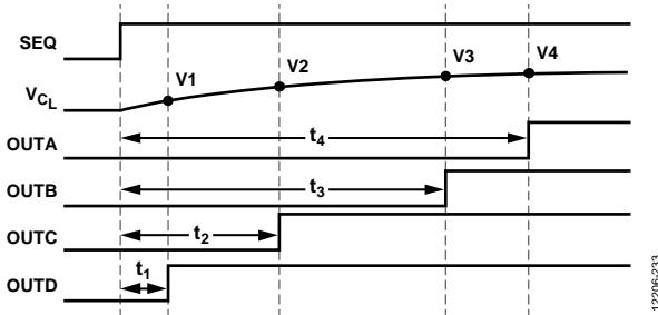
Figure 33. Programmable Sequencing Control Circuit Timing Diagram
