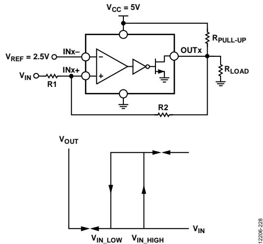
Figure 28. Noninverting Comparator Configuration with Hysteresis
