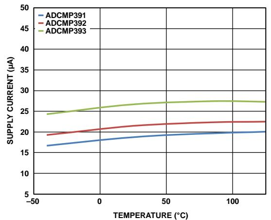
Figure 17. Supply Current vs. Temperature at Output Low Voltage for Various Supply Voltages ( $V_{CC}$ )
