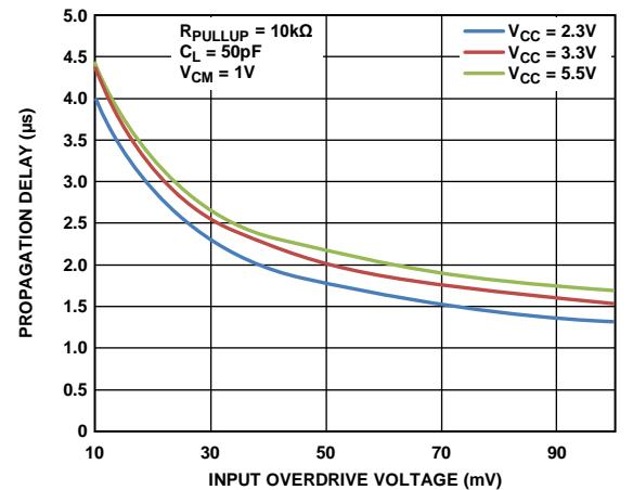
Figure 24. Propagation Delay vs. Input Overdrive Voltage, High to Low, ADCMP392 Channel B
