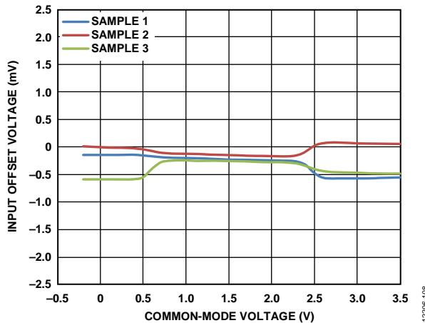
Figure 8. Input Offset Voltage ( $V_{os}$ ) vs. Common-Mode Voltage ( $V_{cm}$ ),
