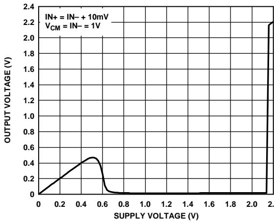
Figure 12. Output Voltage ( $V_{out}$ ) vs. Supply Voltage ( $V_{cc}$ ),  $R_{PULLUP} = 10\text{ k}\Omega$
