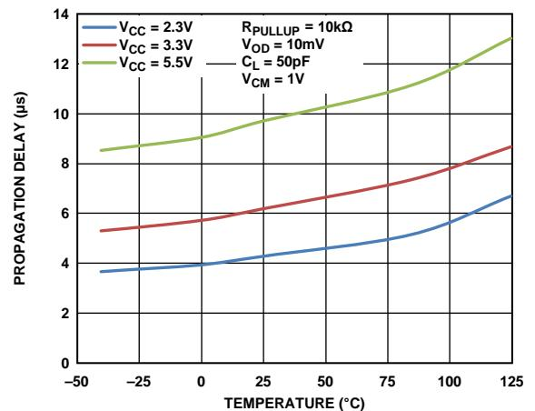
Figure 19. Propagation Delay vs. Temperature, High to Low,  $V_{OD} = 10\text{ mV}$
