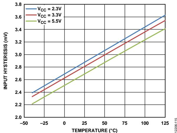
Figure 15. Input Hysteresis vs. Temperature for Various Supply Voltages ( $V_{CC}$ ),  $V_{CM} = 1\text{ V}$
