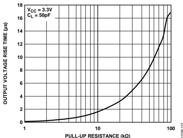
Figure 22. Output Voltage Rise Time ( $t_r$ ) vs. Pull-Up Resistance ( $R_{PULLUP}$ )
