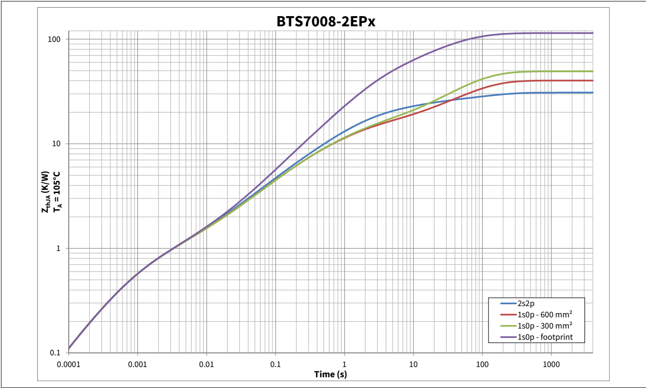
Figure 9 Typical Thermal Impedance. PCB setup according Chapter 4.4.1
