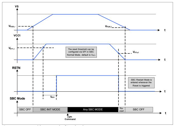
Figure 41 Ramp up / down example of Supply Voltage
