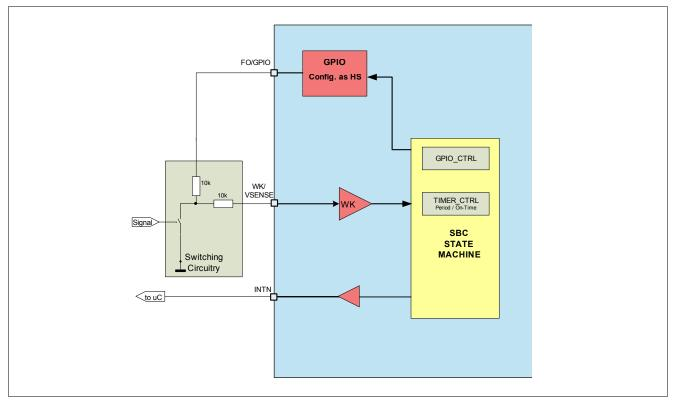
Figure 6 Cyclic Sense Working Principle
