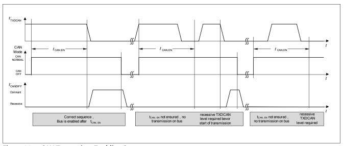
Figure 26 CAN Transceiver Enabling Sequence
