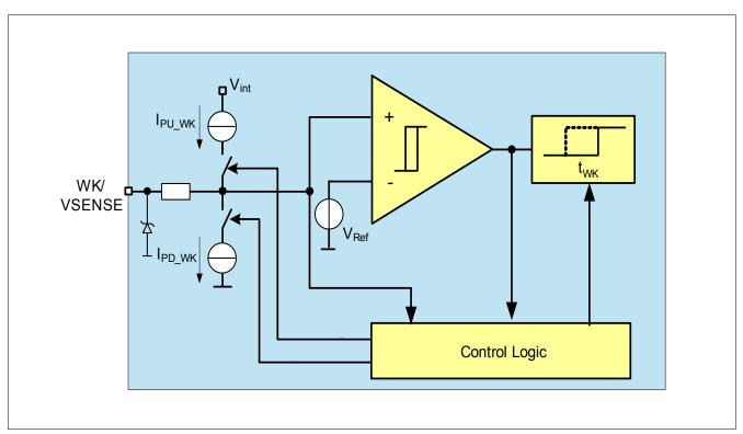
Figure 30 Wake Input Block Diagram
