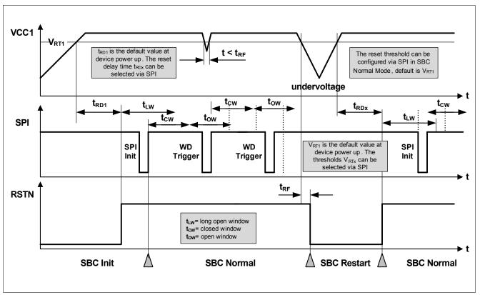
Figure 37 Reset Timing Diagram
