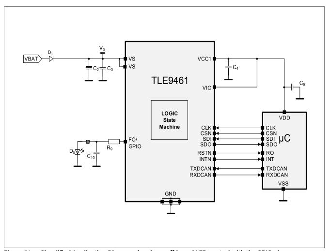
Figure 51 Simplified Application Diagram showing a off-board LED control with the GPIO pin
