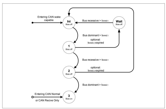
Figure 27 CAN Wake-up Pattern Detection according to the Definition in ISO 11898-2
