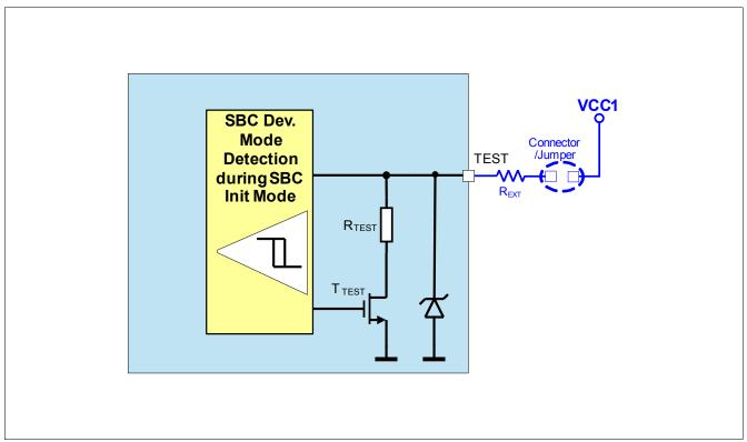
Figure 53 Increasing the Robustness of the pin TEST during Debugging or Programming
