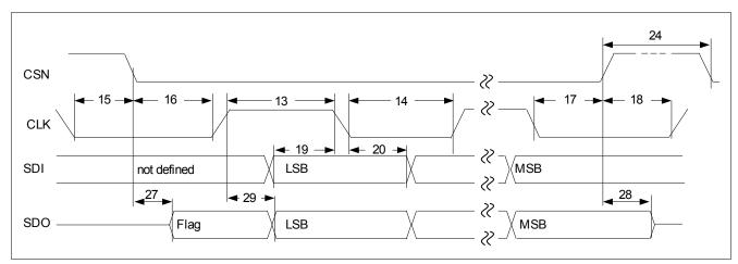
Figure 49 SPI Timing Diagram
