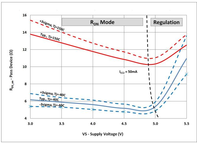
Figure 22 On-resistance range of VCC2 pass device during linear (R<sub>ON</sub>) mode for /<sub>CC2</sub> = 50mA
