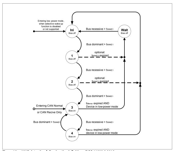
Figure 16 WUP detection following the definition of ISO 11898-2:2016
