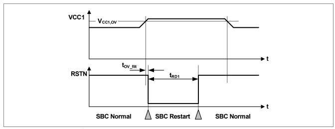
Figure 43 VCC1 Over Voltage Timing Diagram
