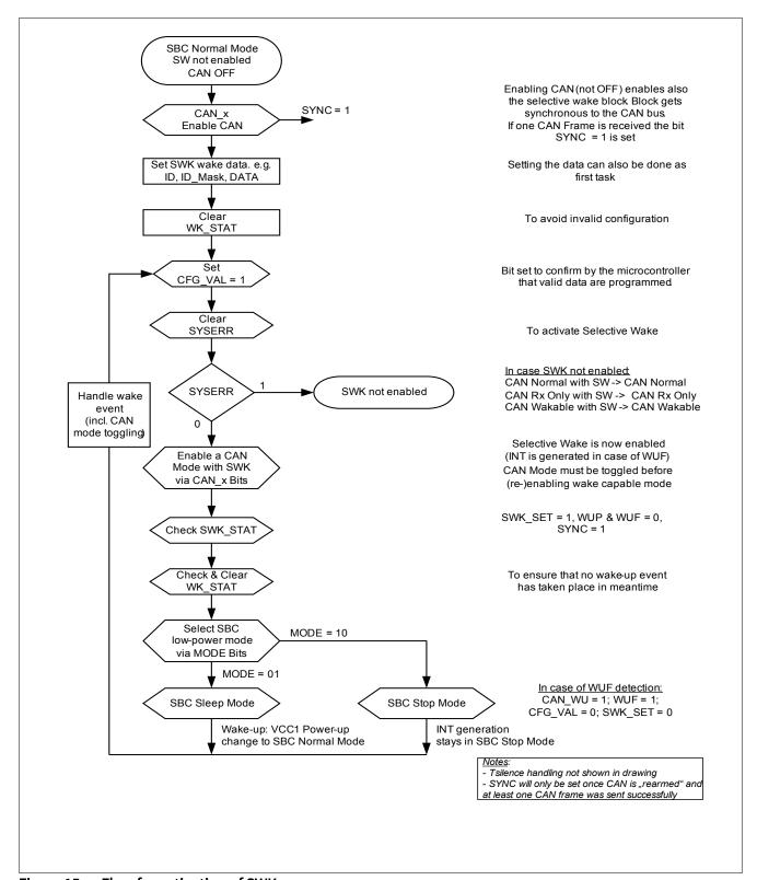
Figure 15 Flow for activation of SWK
