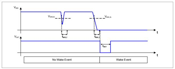
Figure 31 Wake-up Filter Timing for Static Sense
