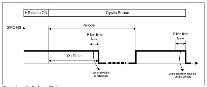
Figure 8 Cyclic Sense Timing
