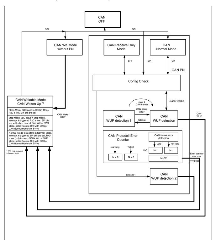
Figure 14 **CAN Selective Wake State Diagram**
