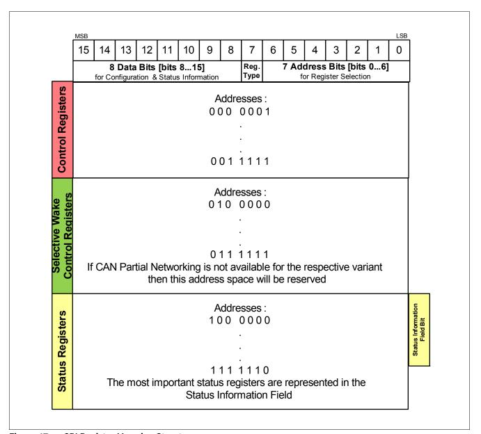
**SPI Register Mapping Structure** Figure 47
