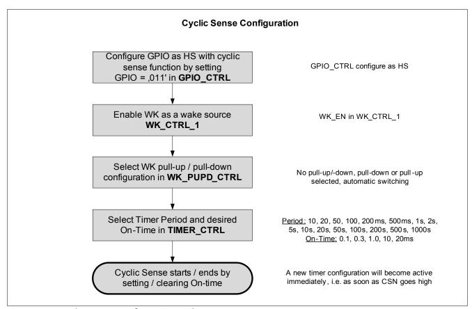
Figure 7 Cyclic Sense: Configuration and Sequence
