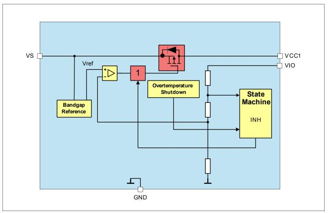
Figure 19 Module Block Diagram
