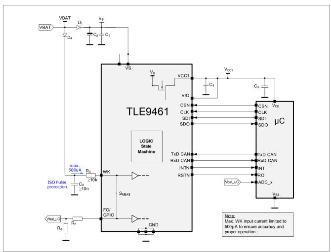
Figure 52 Simplified Application Diagram showing the Alternate High-Voltage Measurement Function via WK/SENSE and FO/GPIO
