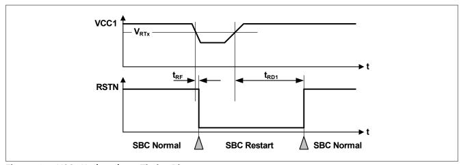
Figure 42 VCC1 Undervoltage Timing Diagram
