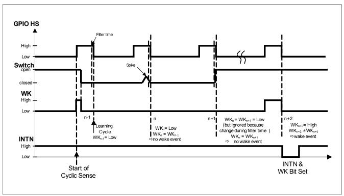
Cyclic Sense Example Timing for SBC Stop Mode, HS starts Low, GND based WK/VSENSE input Figure 9
