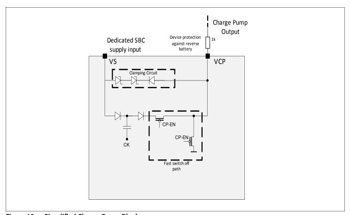
Figure 12 Simplified Charge Pump Block
