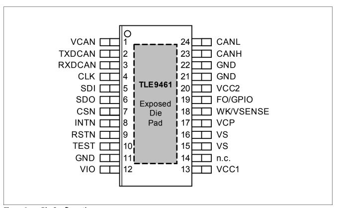
Figure 2 Pin Configuration
