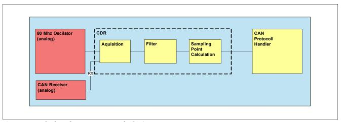
Figure 18 Clock and Data Recovery Block Diagram
