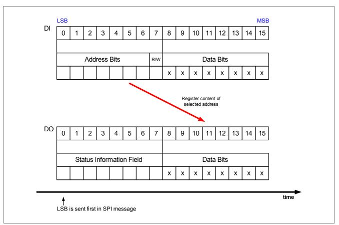
Figure 45 SPI Operation Mode
