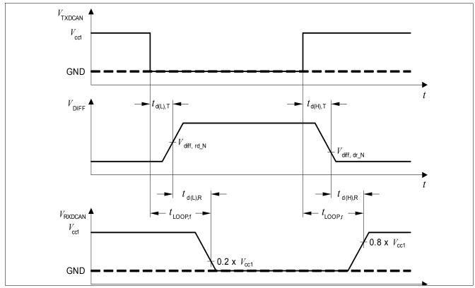
Figure 28 Timing Diagrams for Dynamic Characteristics
