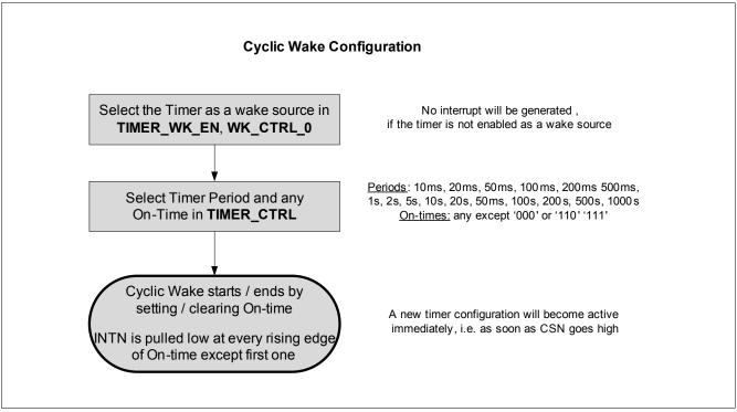
Figure 11 Cyclic Wake: Configuration and Sequence
