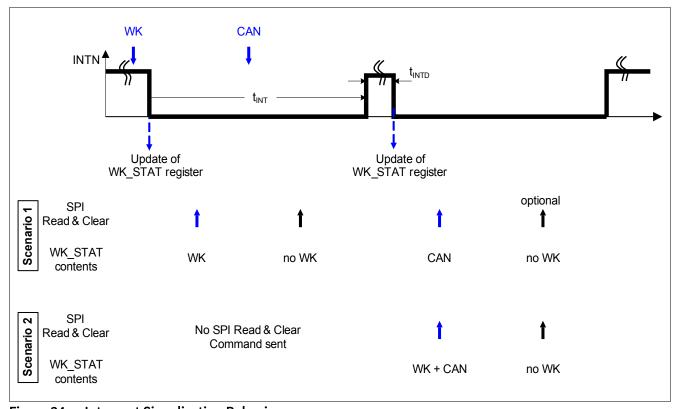
Figure 34 Interrupt Signalization Behavior
