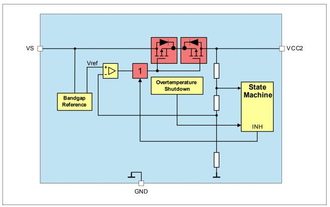
Figure 20 Module Block Diagram
