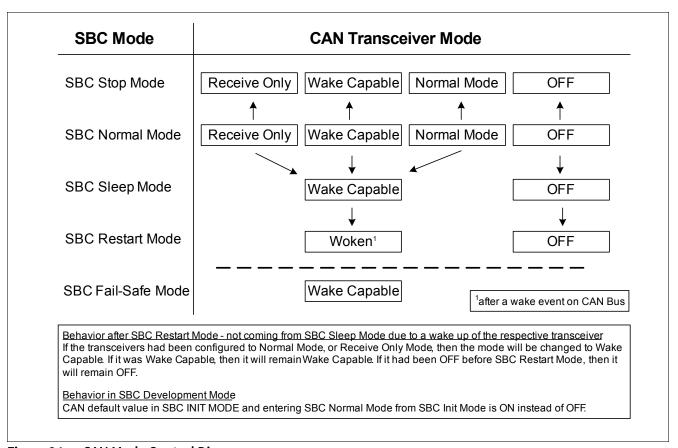
Figure 24 CAN Mode Control Diagram
