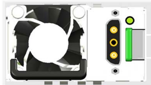
DC Power Cable Connectors
