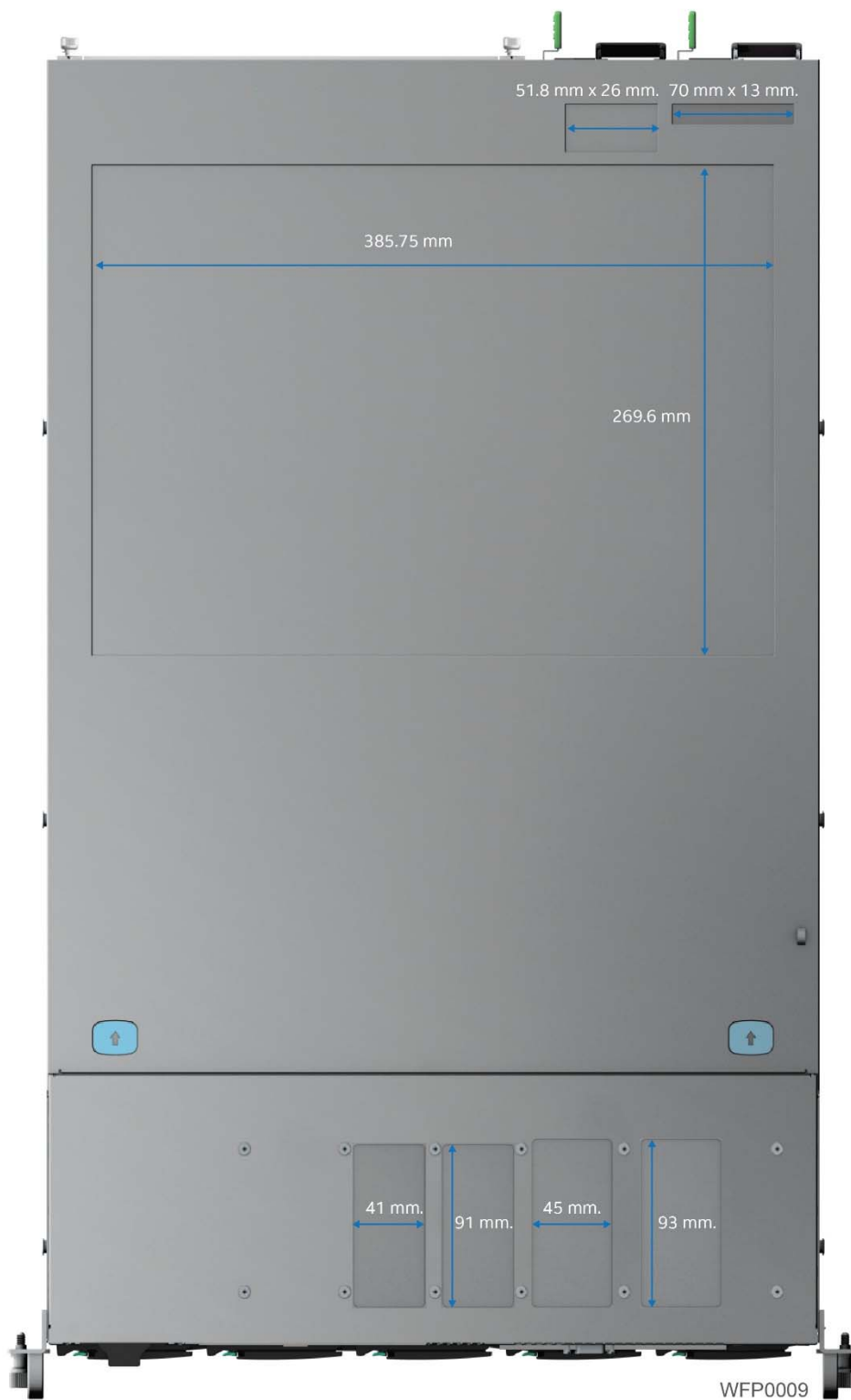
Figure 17. Label emboss dimensions
