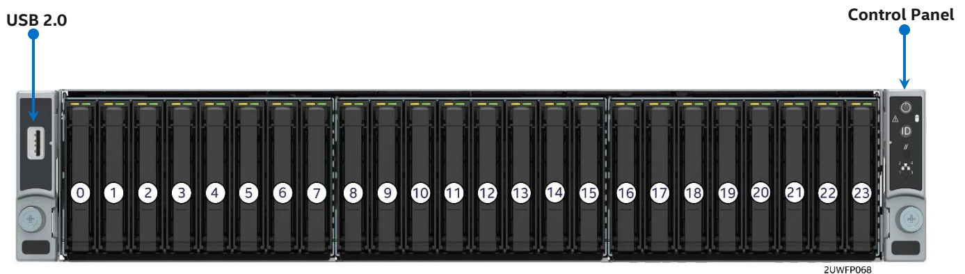
Figure 40. 2.5" front mount drive bay, 24 drive (R2224WFxxx) configuration
