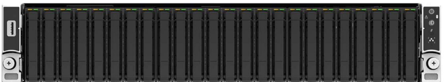
Figure 14. 2.5" x 24 front drive bay configuration – R2224WFxxxx
