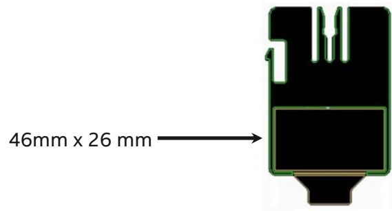
Figure 18. Pull-out tab label emboss dimensions, non-storage models
