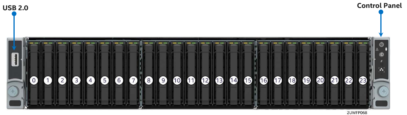
Figure 40. 2.5" front mount drive bay, 24 drive (R2224WFxxx) configuration
