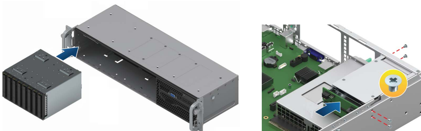
Figure 48. 2.5" drive bay module placement options
