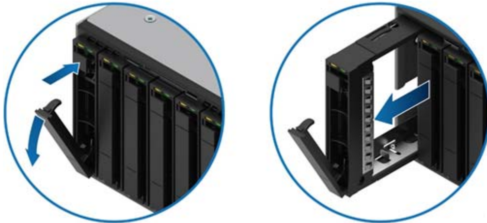
Figure 43. Drive carrier removal
