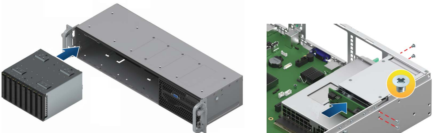
Figure 48. 2.5" drive bay module placement options
