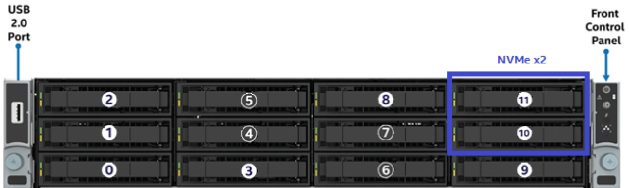
Figure 42. 3.5" drive bay, 12 drive configuration
