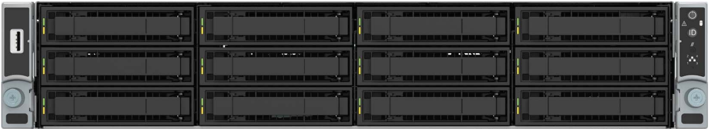
Figure 10. 3.5" x 8 front drive bay configuration – R2308WFxxxx
