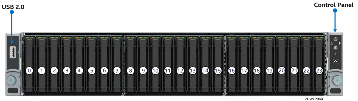
Figure 40. 2.5" front mount drive bay, 24 drive (R2224WFxxx) configuration
