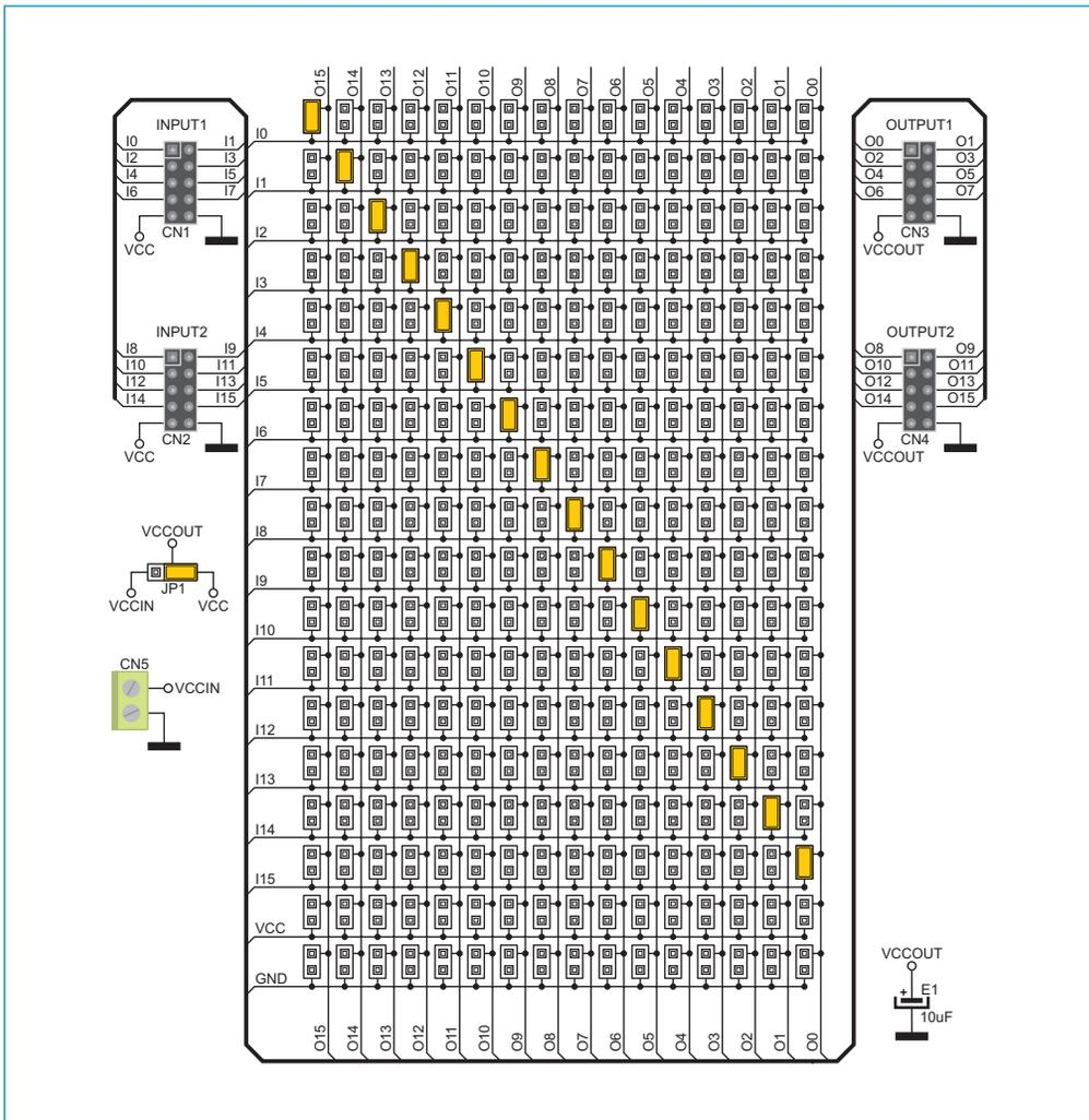
Figure 4: Smart ADAPT2 board connection schematic
