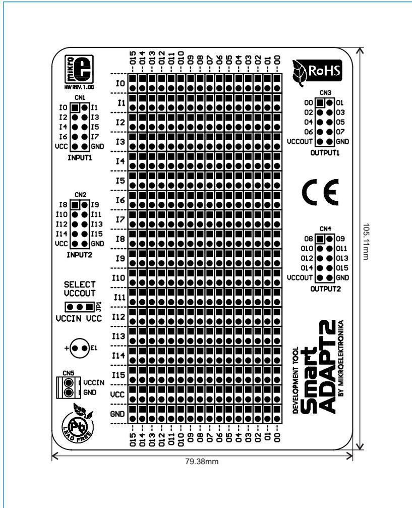
Figure 5: Dimensions of the Smart ADAPT2 board
