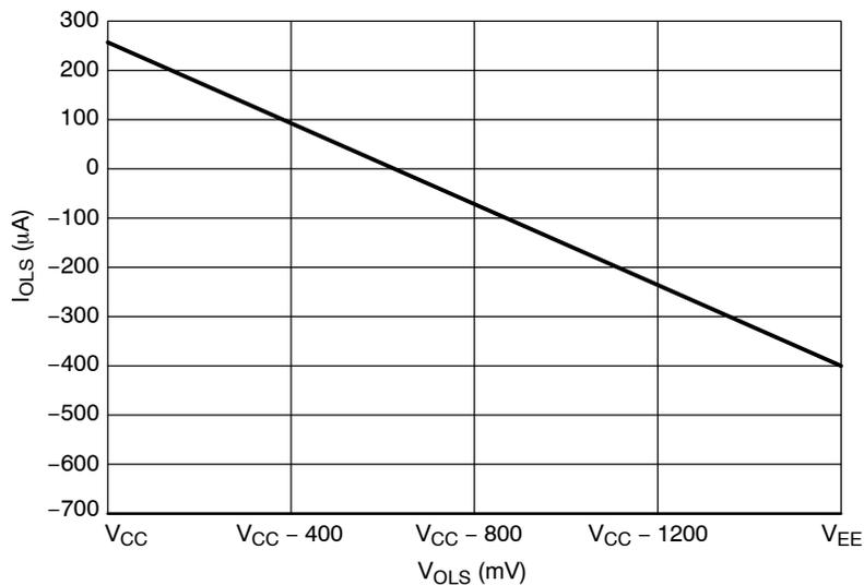
**Figure 10. Typical OLS Input Current vs. OLS Input Voltage**
