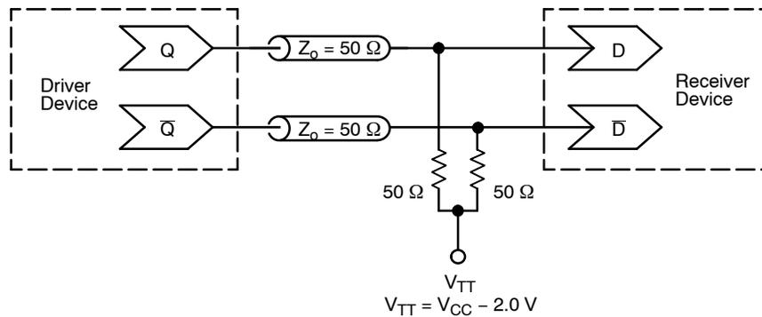
Figure 13. Typical Termination for Output Driver and Device Evaluation
