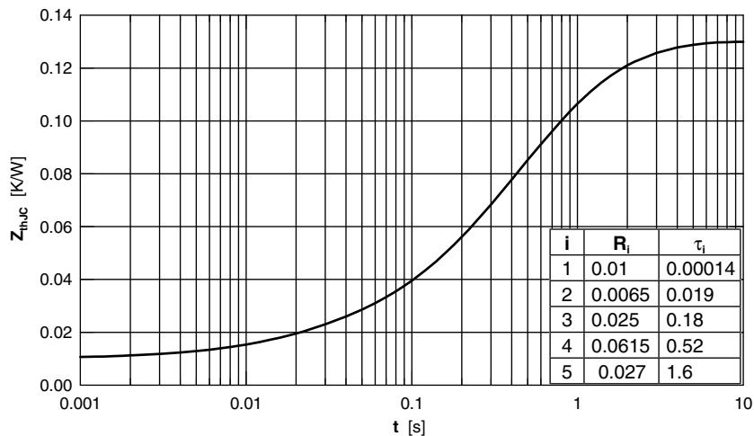
Fig. 8 Transient thermal impedance junction to case
