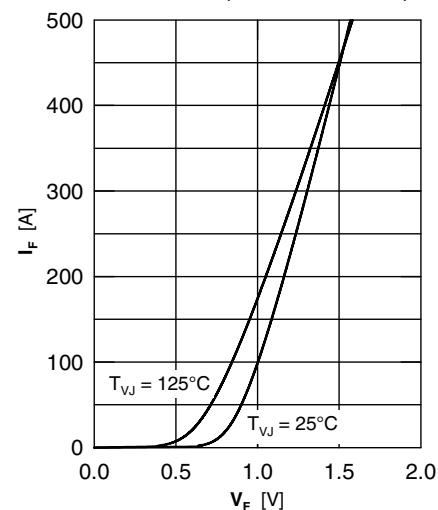
Fig. 7 Forward current versus voltage drop
