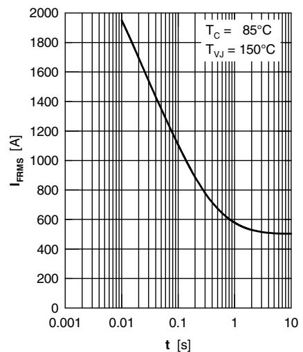
Fig. 5 Rated RMS current versus time (360° conduction)
