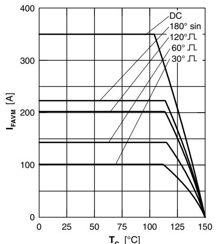
Fig. 3 Maximum forward current at case temperature
