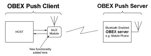
The Obex Push profile implementation provides the capability to a host to act as a 'Obex Push client' to a peer device providing an 'obex push server' profile.
