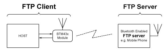
An FTP client capability implies the ability to send and receive files and also to manipulate file objects in the remote device. The Bluetooth FTP server profile specification describes the profile as one built on Obex Exchange (OBEX) which is in turn built on SPP.
