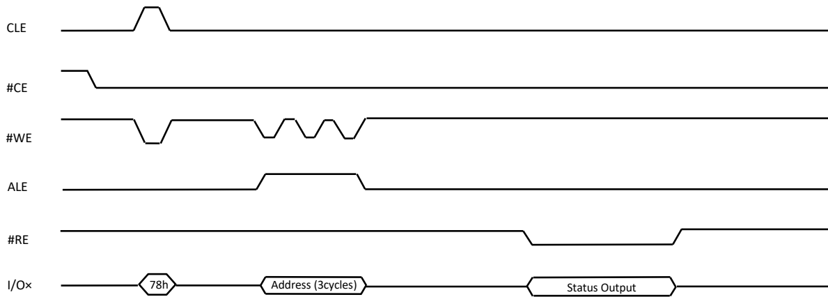
Figure 9-8 Read Status Enhanced (78h) Operation
