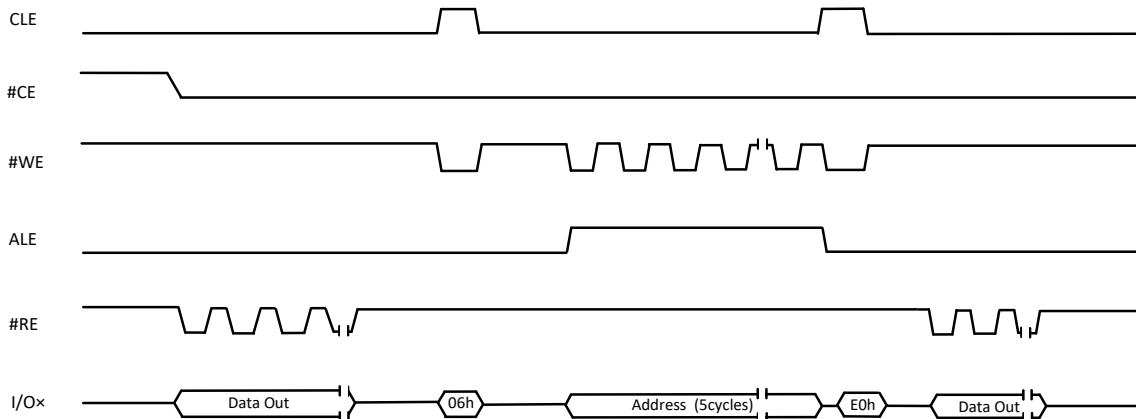
Figure 9-4 Two Plane Random Data Read (06h-E0h) Operation
