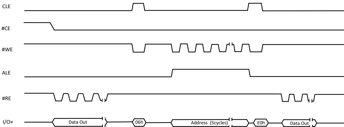
Figure 9-4 Two Plane Random Data Read (06h-E0h) Operation
