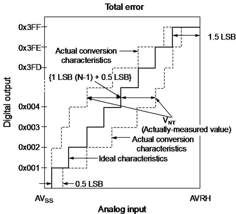
$$1\text{LSB} (\text{Ideal value}) = \frac{\text{AVRH} - \text{AV}_{\text{ss}}}{1024} [\text{V}]$$
