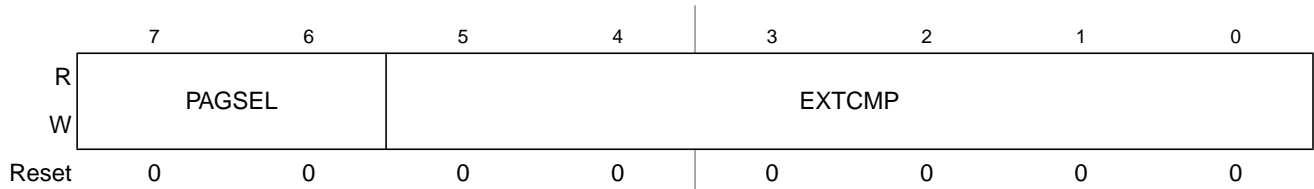
Figure 7-15. Debug Comparator A Extended Register (DBGCAx)
