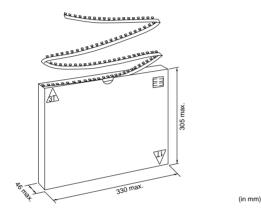
■ Dimensions of Magazine Packaging PV01 PVC6 370 +0 9.0±0.5 413 +0 9.8±0.5 15.3±0.5 18.8±0.5 PV36W/Y/X/Z PV36P 508 <sup>+0</sup><sub>-1.0</sub> 11.5±0.5 508 <sup>+0</sup><sub>-1.0</sub> 21.1±0.5 18.0±0.5 (in mm)
