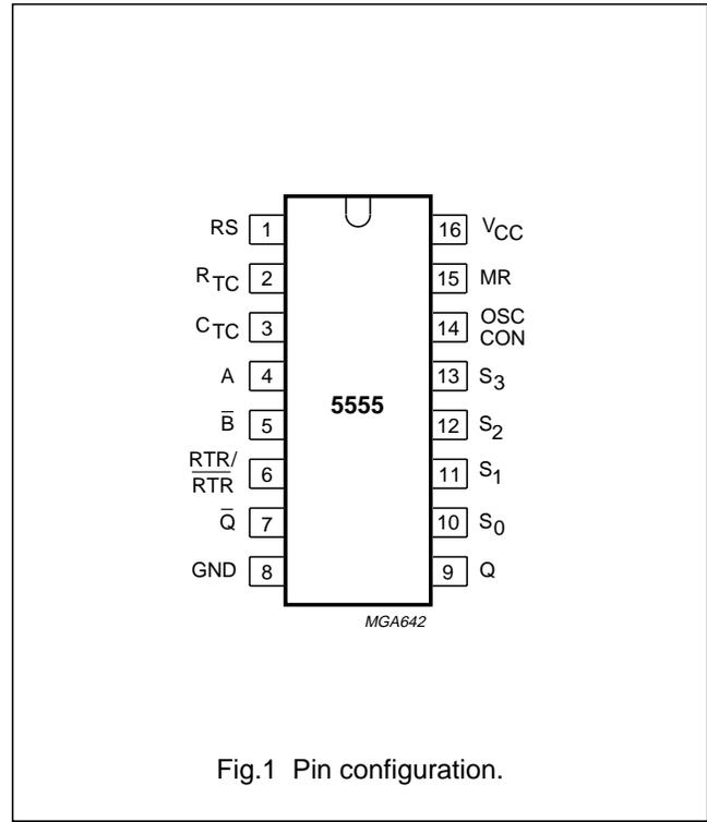
Fig.1 Pin configuration.
