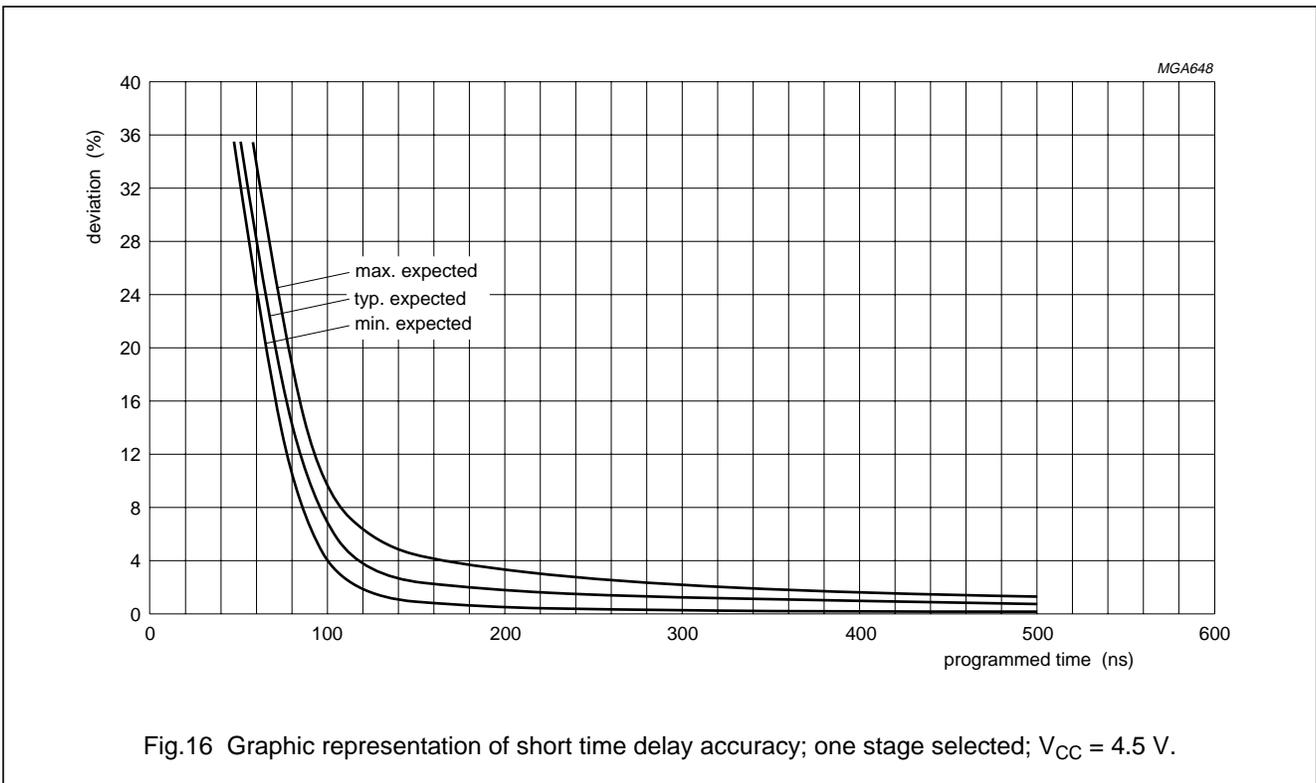
Fig.16 Graphic representation of short time delay accuracy; one stage selected;  $V_{CC} = 4.5$  V.
