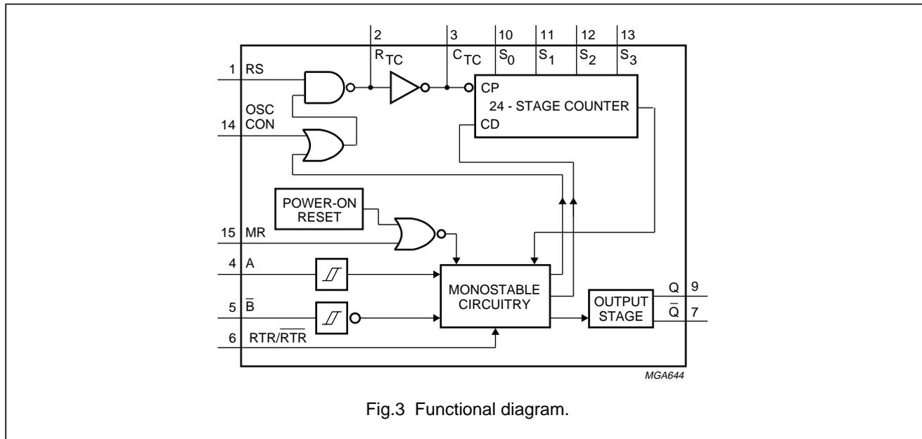
Fig.3 Functional diagram.
