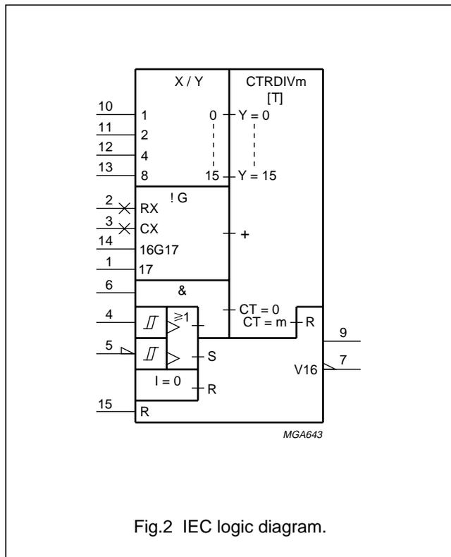
Fig.2 IEC logic diagram.
