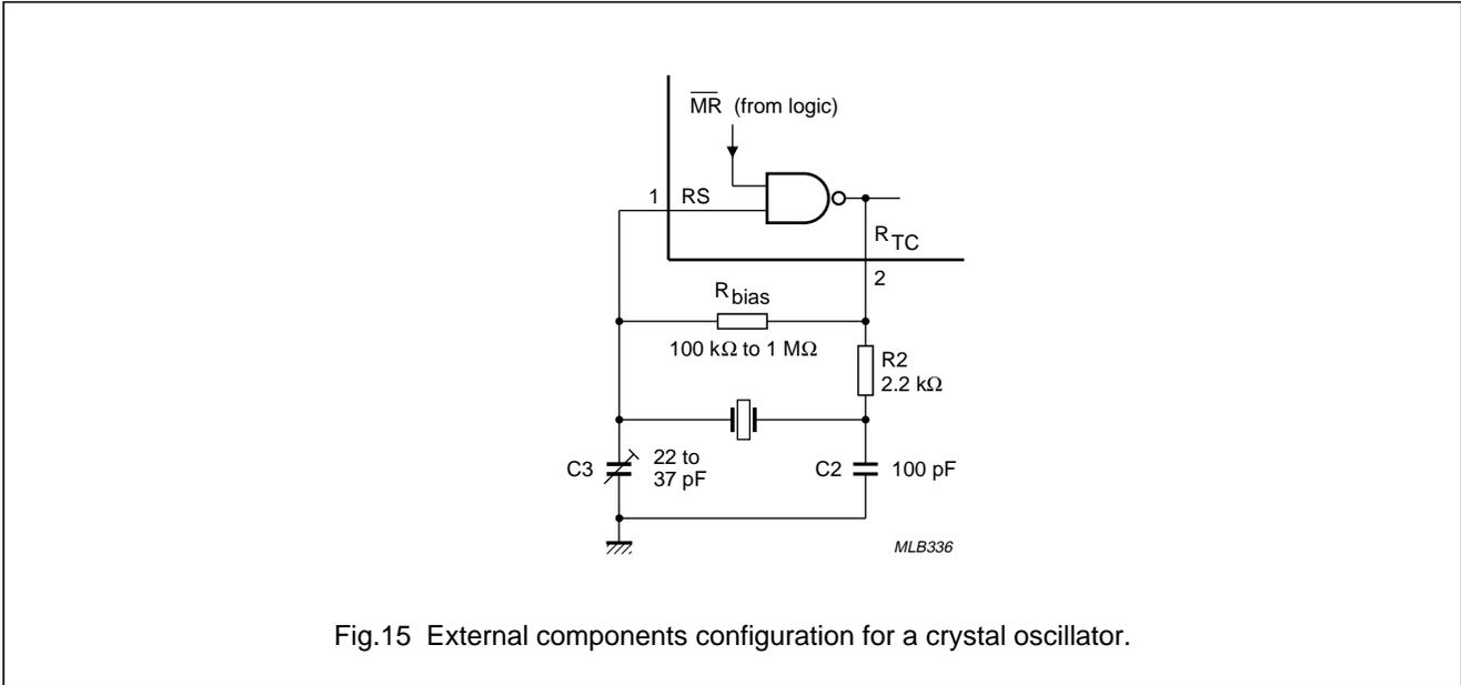
Fig.15 External components configuration for a crystal oscillator.
