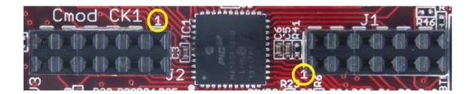
See the attached pinout diagram and tables in the appendices for more information about connecting peripheral modules and other devices to the chipKIT Cmod. These tables describe the mapping between pins on the PIC32MX150F128D microcontroller and the pins on the connectors.
