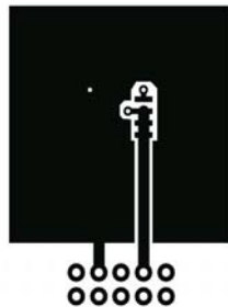
a) 50 ^{\circ}\text{C}/\text{W} when mounted on a 1 in 2 pad of 2 oz copper.
