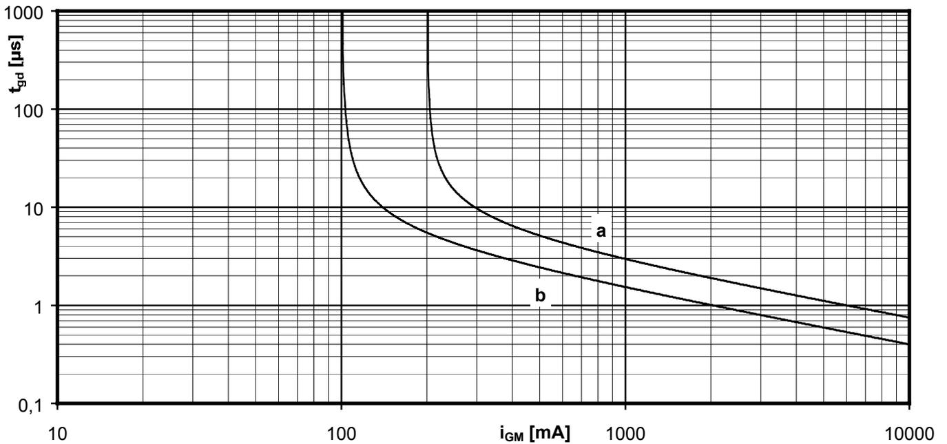
Zündverzug / Gate controlled delay time  $t_{gd} = f(i_G)$
