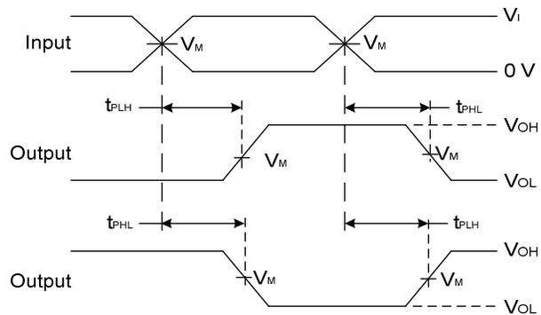
**Voltage Waveform Propagation Delay Times
