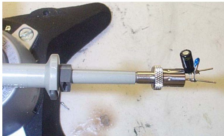
Figure 37 – Oscilloscope Probe with Probe Master ( www.probemaster.com ) 4987A BNC Adapter. (Modified with wires for ripple measurement, and two parallel decoupling capacitors added)
