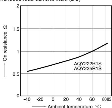
2.- (2) On resistance vs. ambient temperature characteristics
