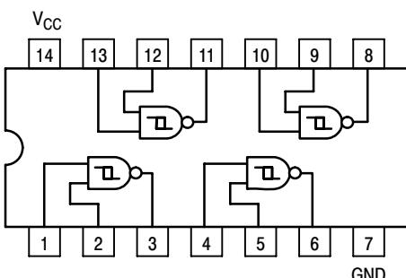
Figure 1. Pinout; 14-Lead Packages Conductors
