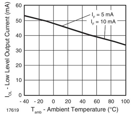
Fig. 14 - Low Level Output Current vs. Ambient Temperature
