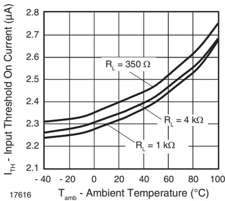
Fig. 11 - Input Threshold On Current vs. Ambient Temperature
