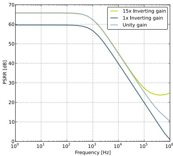
**Figure 4.23. OPAMP Positive Power Supply Rejection Ratio**
