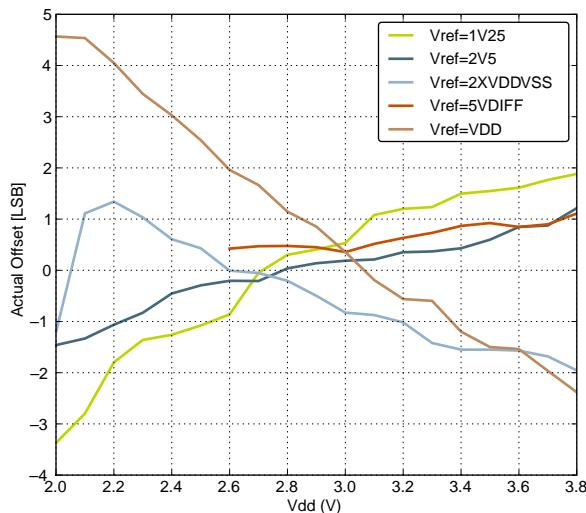
**Offset vs Supply Voltage, Temp = 25 °C**
