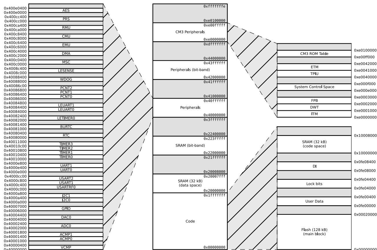
Figure 3.2. EZR32LG230 Memory Map with Largest RAM and Flash Sizes
