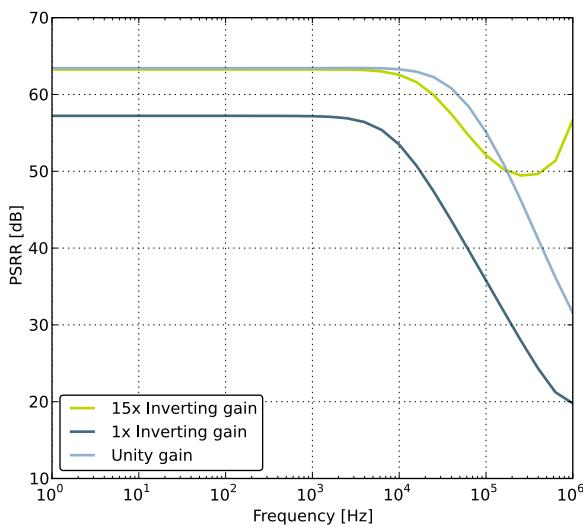
**Figure 4.24. OPAMP Negative Power Supply Rejection Ratio**
