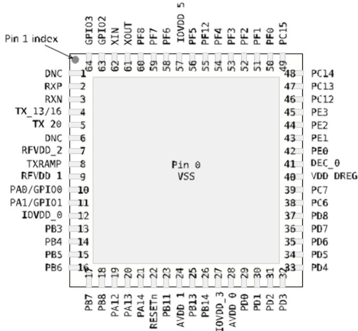
**Figure 5.1. Pinout (top view, not to scale)**
