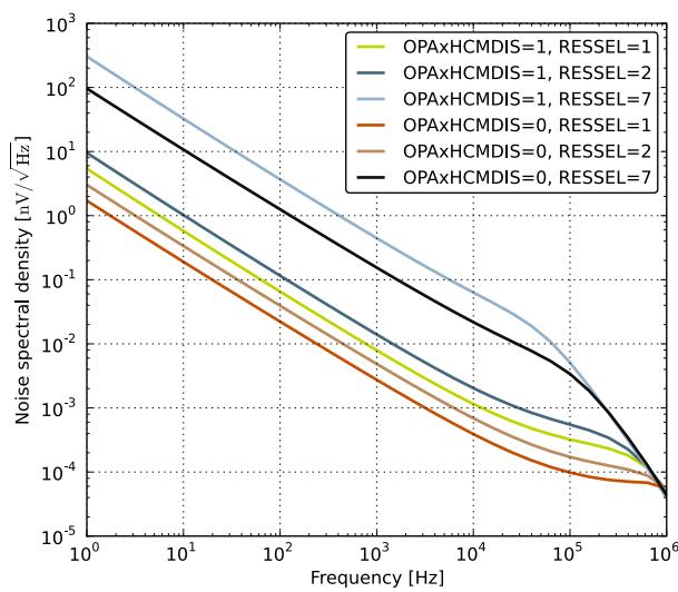
Figure 4.26. OPAMP Voltage Noise Spectral Density (Non-Unity Gain)
