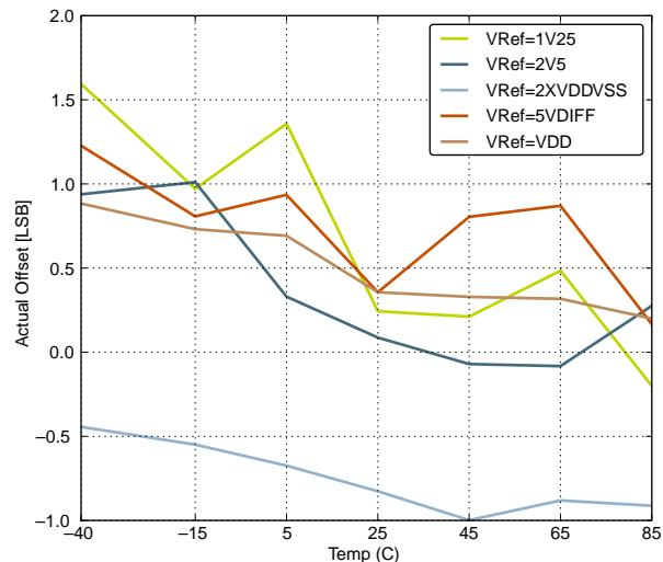
**Offset vs Temperature, V<sub>DD</sub> = 3 V****Figure 4.19. ADC Absolute Offset, Common Mode = V<sub>DD</sub>/2**
