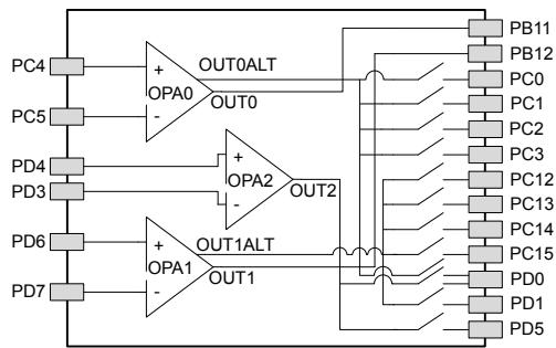
**Figure 5.2. Opamp Pinout**
