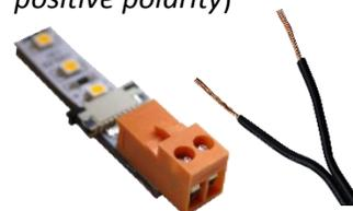
**8** Insert wire (matching polarity) tighten screws and connect to class 2 power source to verify connections, then install LED flex strips as needed
