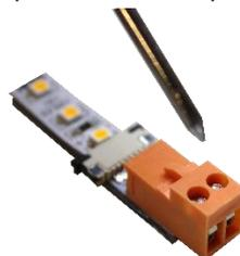
**7** Strip cable back ¼" to expose (+) and (-) wire, (if using Inspired LED cable, white writing indicates positive polarity)
