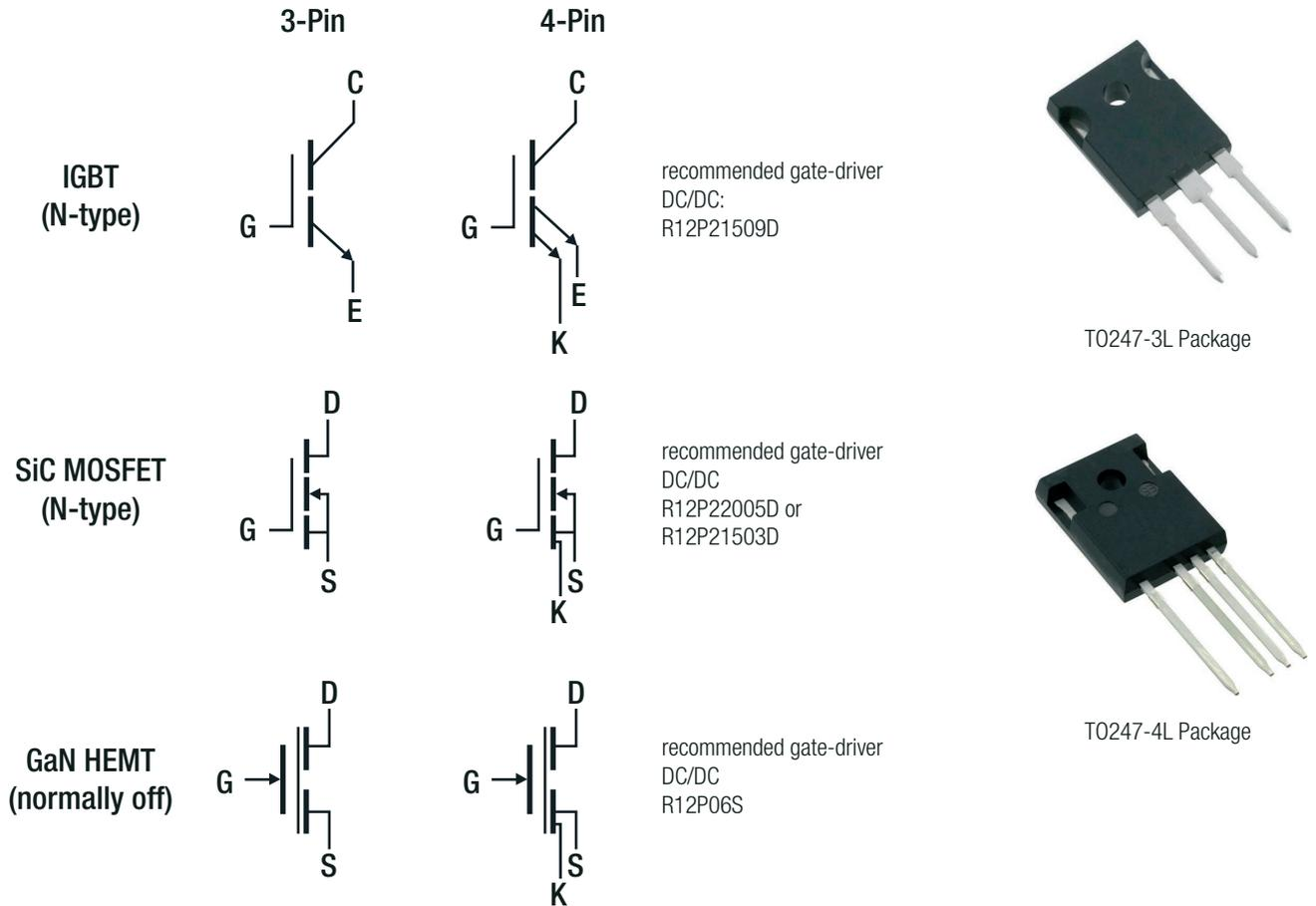
**Important:** using three pin or four pin T0247 packages:
