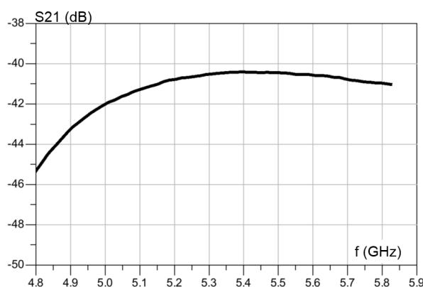
**Figure 6. Attenuation 3f0 (dB)**
