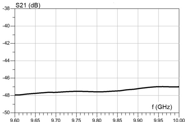
**Figure 8. Attenuation 5f0 (dB)**
