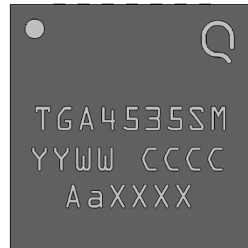
28 lead 5x5mm QFN package
