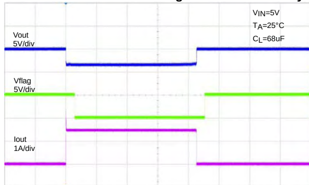
Short Circuit with Blanking Time and Recovery
