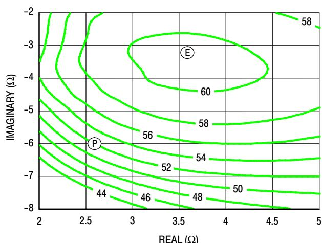
Figure 11. P1dB Load Pull Efficiency Contours (%)
