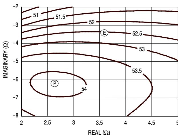
Figure 14. P3dB Load Pull Output Power Contours (dBm)
