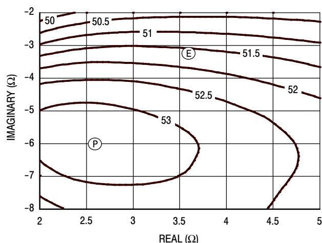
Figure 10. P1dB Load Pull Output Power Contours (dBm)
