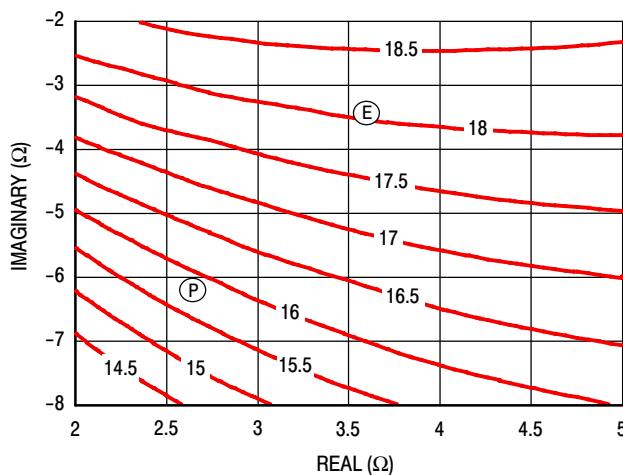
Figure 16. P3dB Load Pull Gain Contours (dB)
