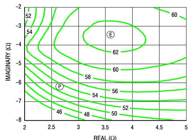
Figure 15. P3dB Load Pull Efficiency Contours (%)
