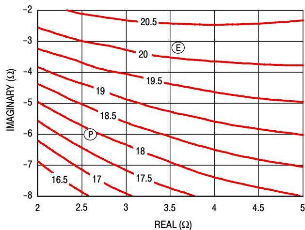
Figure 12. P1dB Load Pull Gain Contours (dB)
