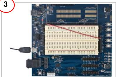
1. Place a jumper on J12 and another between  $V_{DD}$  and  $V_{REG}$  on J2.
