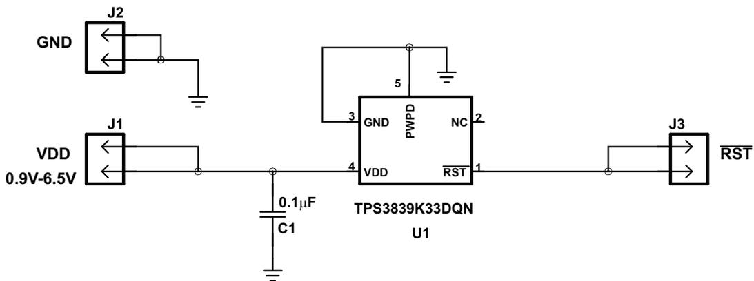
Figure 4. TPS3839K33EVM-112 Schematic
