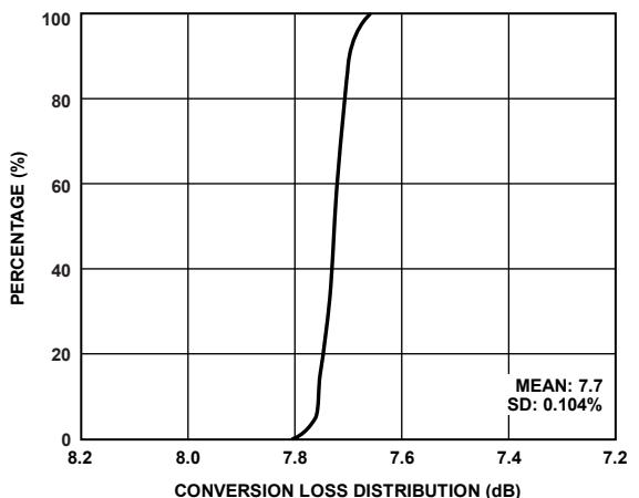
Figure 24. Conversion Loss Distribution
