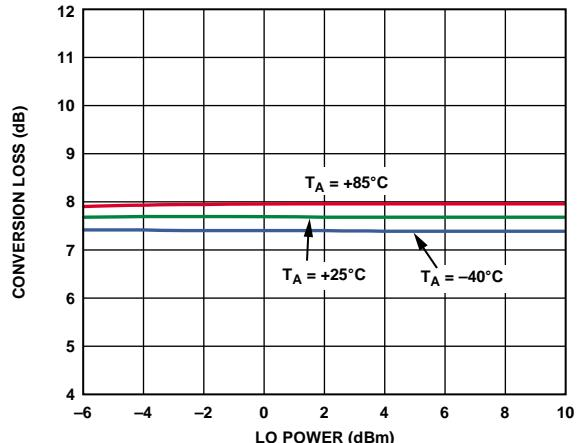
Figure 18. Power Conversion Loss vs. LO Power
