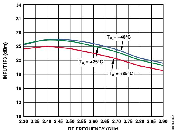
Figure 39. Input IP3 vs. RF Frequency at 3.3 V
