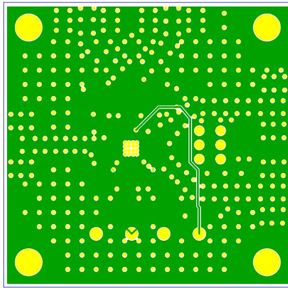
Figure 51. Evaluation Board Power Plane, Internal Layer 2
