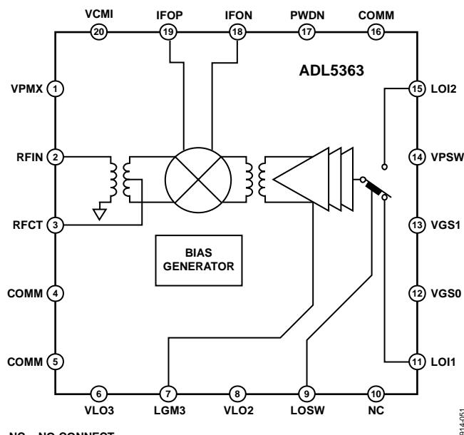
Figure 46. Simplified Schematic
