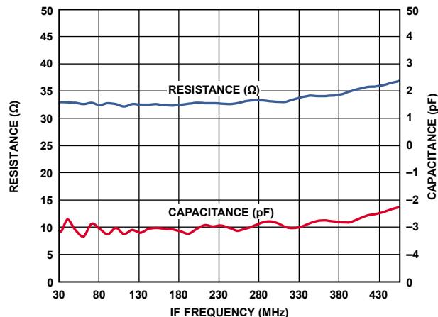
Figure 26. IF Output Impedance ( $R$  Parallel,  $C$  Equivalent)
