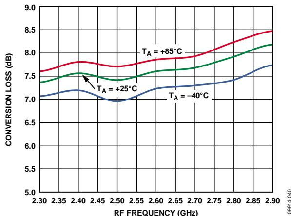
Figure 38. Power Conversion Loss vs. RF Frequency at 3.3 V
