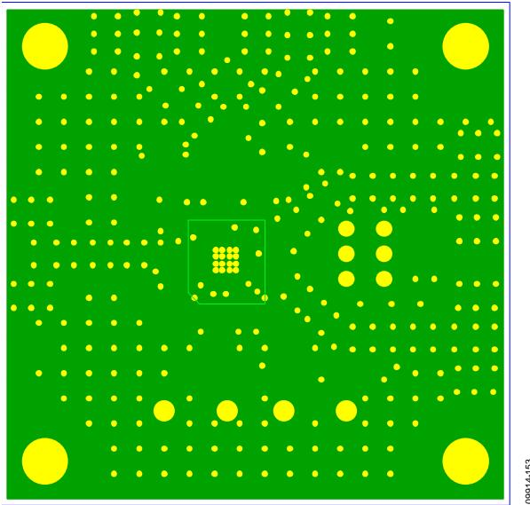
Figure 50. Evaluation Board Ground Plane, Internal Layer 1
