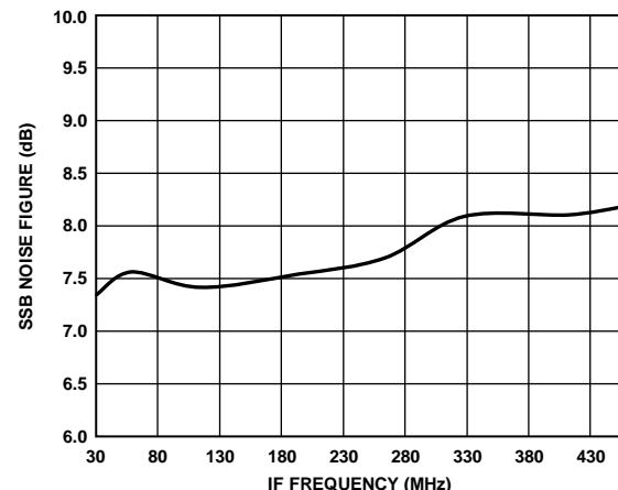
Figure 17. SSB Noise Figure vs. IF Frequency
