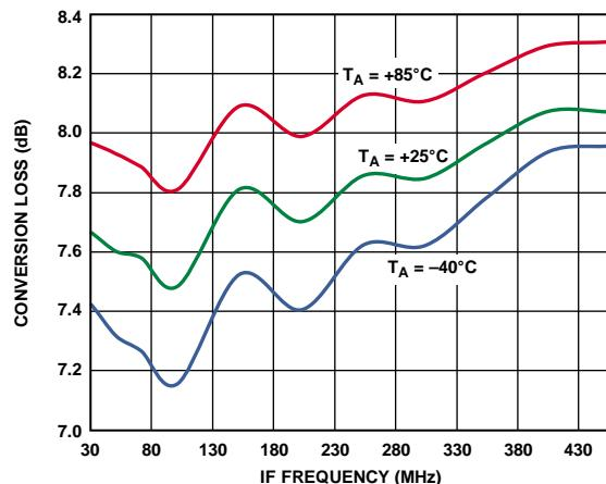
Figure 14. Power Conversion Loss vs. IF Frequency
