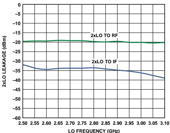
Figure 33. 2LO Leakage vs. LO Frequency
