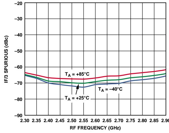
Figure 22. IF/3 Spurious vs. RF Frequency
