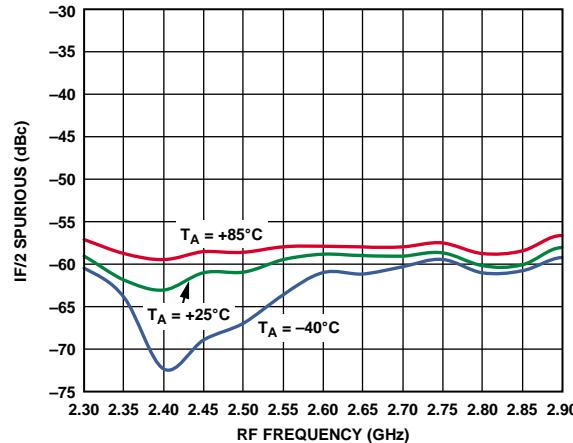
Figure 21. IF/2 Spurious vs. RF Frequency
