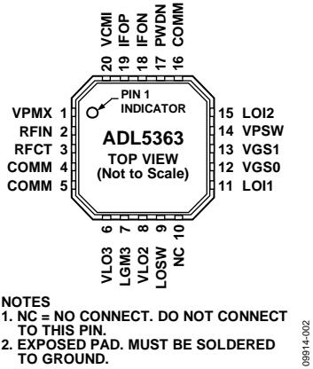
Figure 2. Pin Configuration
