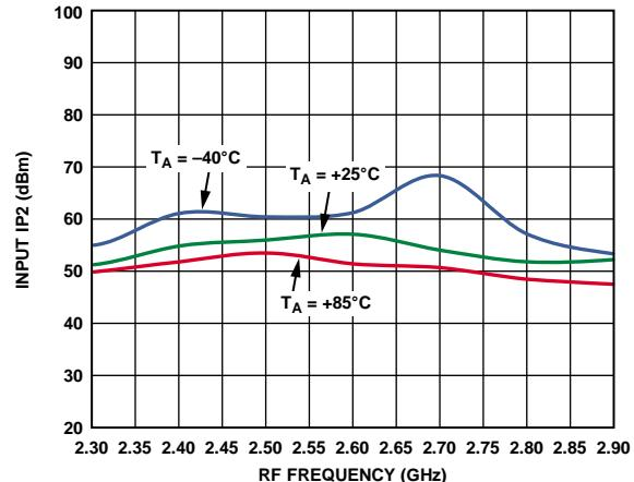
Figure 40. Input IP2 vs. RF Frequency at 3.3 V
