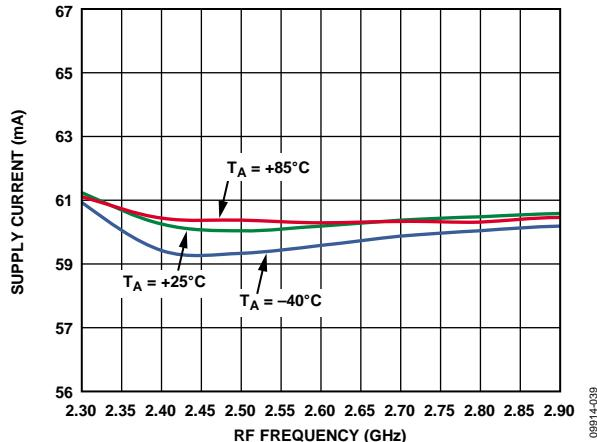
Figure 37. Supply Current vs. RF Frequency at 3.3 V
