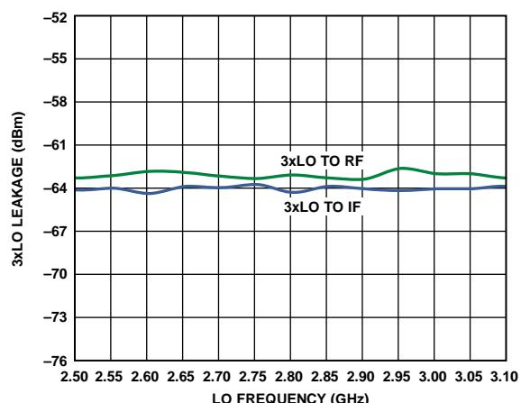
Figure 34. 3LO Leakage vs. LO Frequency
