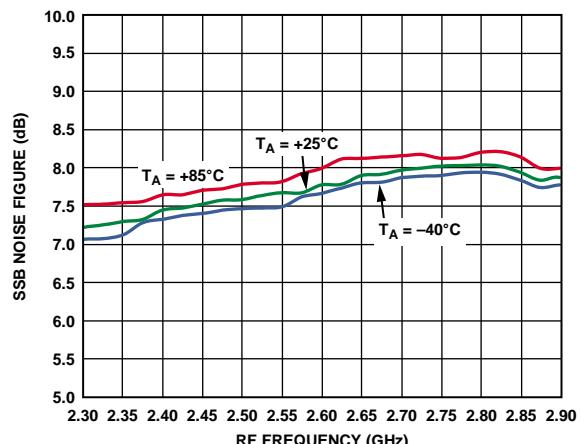
Figure 7. SSB Noise Figure vs. RF Frequency
