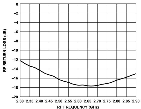
Figure 27. RF Port Return Loss, Fixed IF
