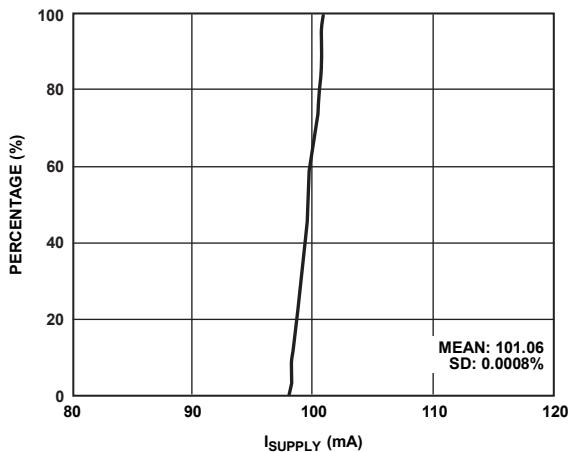
Figure 23. Supply Current Distribution
