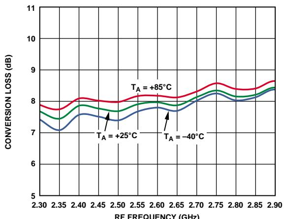
Figure 4. Power Conversion Loss vs. RF Frequency
