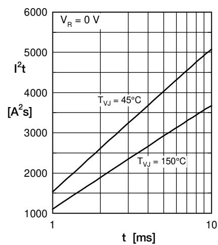
Fig. 3  $I^2t$  vs. time per diode
