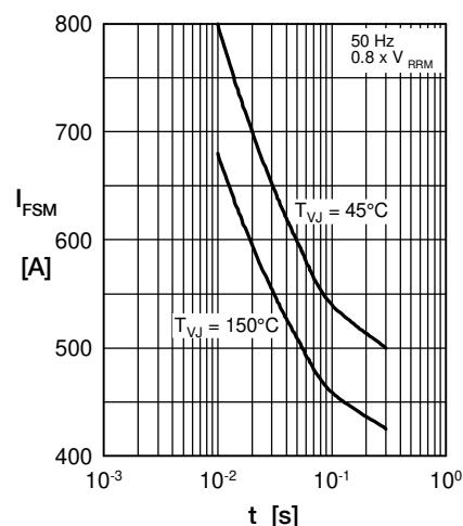
Fig. 2 Surge overload current vs. time per diode
