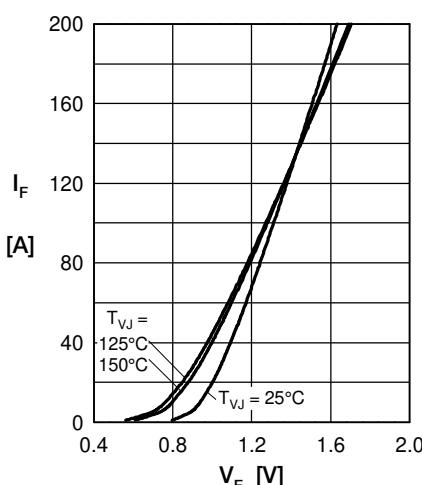
Fig. 1 Forward current vs. voltage drop per diode
