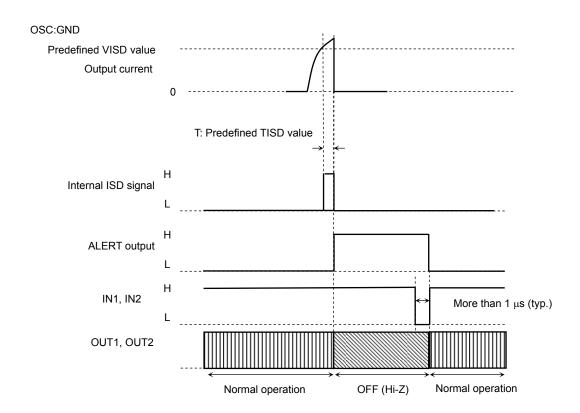
Note: The ISD circuit is activated if the absolute maximum current rating is violated. Note that the circuit is provided as an auxiliary only and does not necessarily provide the IC with a perfect protection from damages due to overcurrent caused by power fault, ground fault, load-short and the like.
