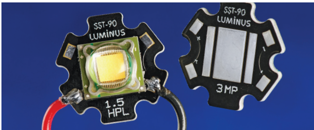
Wire soldering on THERMAL CLAD.
