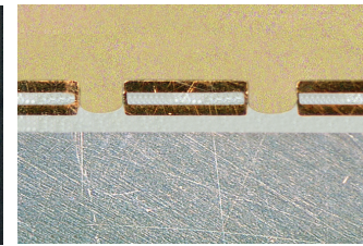
Henkel has the ability to laminate heavy copper up to 5 oz. (175µm) finished on the internal layer utilizing a thicker deposit of HT dielectric.
