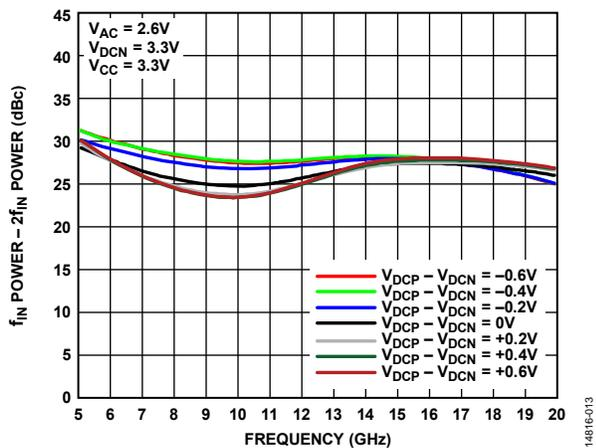
Figure 13.  $f_{IN}$  Power -  $2f_{IN}$  Power vs. Frequency
