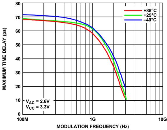
Figure 31. Maximum Time Delay vs. Modulation Frequency, Input Data Rate = 22.5 Gbps, PRBS 2<sup>33</sup> - 1, 6 dBm Input Power Applied to V<sub>DCP</sub> and V<sub>DCN</sub> Terminated to 50 Ω
