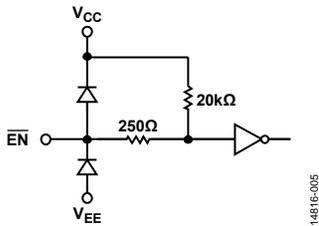
Figure 5. EN Interface Schematic
