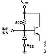
Figure 4. INP and INN Interface Schematic
