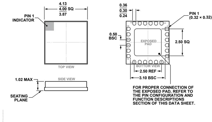
Figure 36. 24-Terminal Ceramic Leadless Chip [LCC] (E-24-1)
