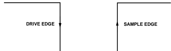
Figure 66. SPI Mode 3, SCLK Edges
